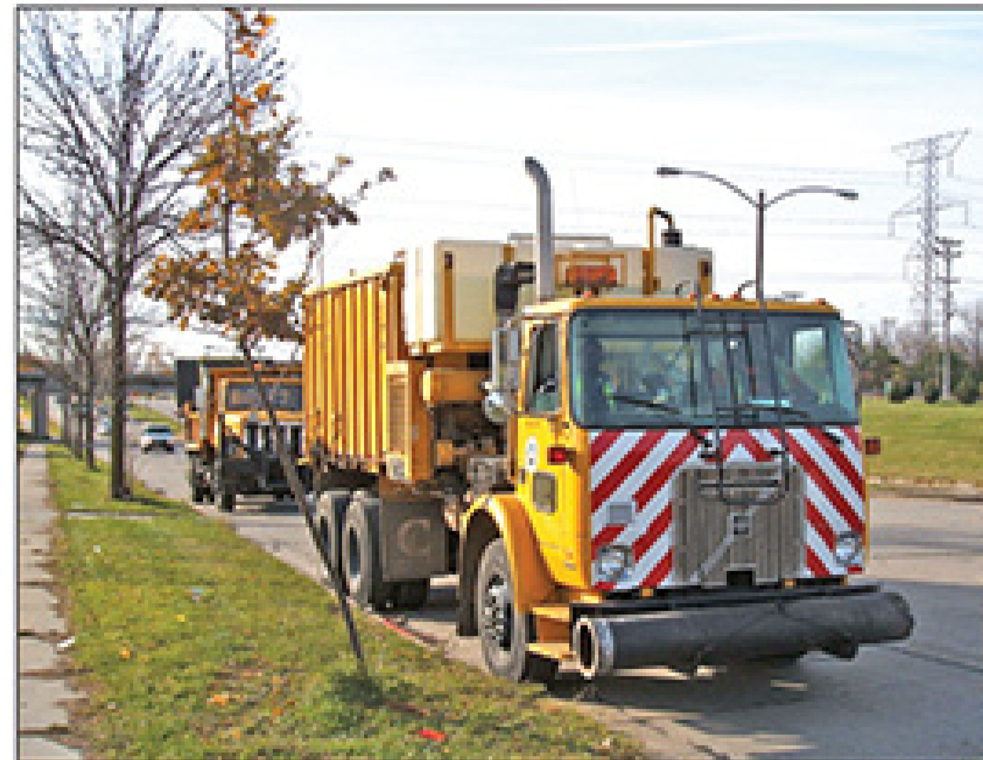
Left, one of the Milwaukee County Highway Department's VacAll trucks waits at an intersection to start a catch-basin cleaning project. Below, highway maintenance supervisor Derwin Pottinger and team members (from left) Bill Luzinski, Tony Minter and Oscar Rush clean the basin.
