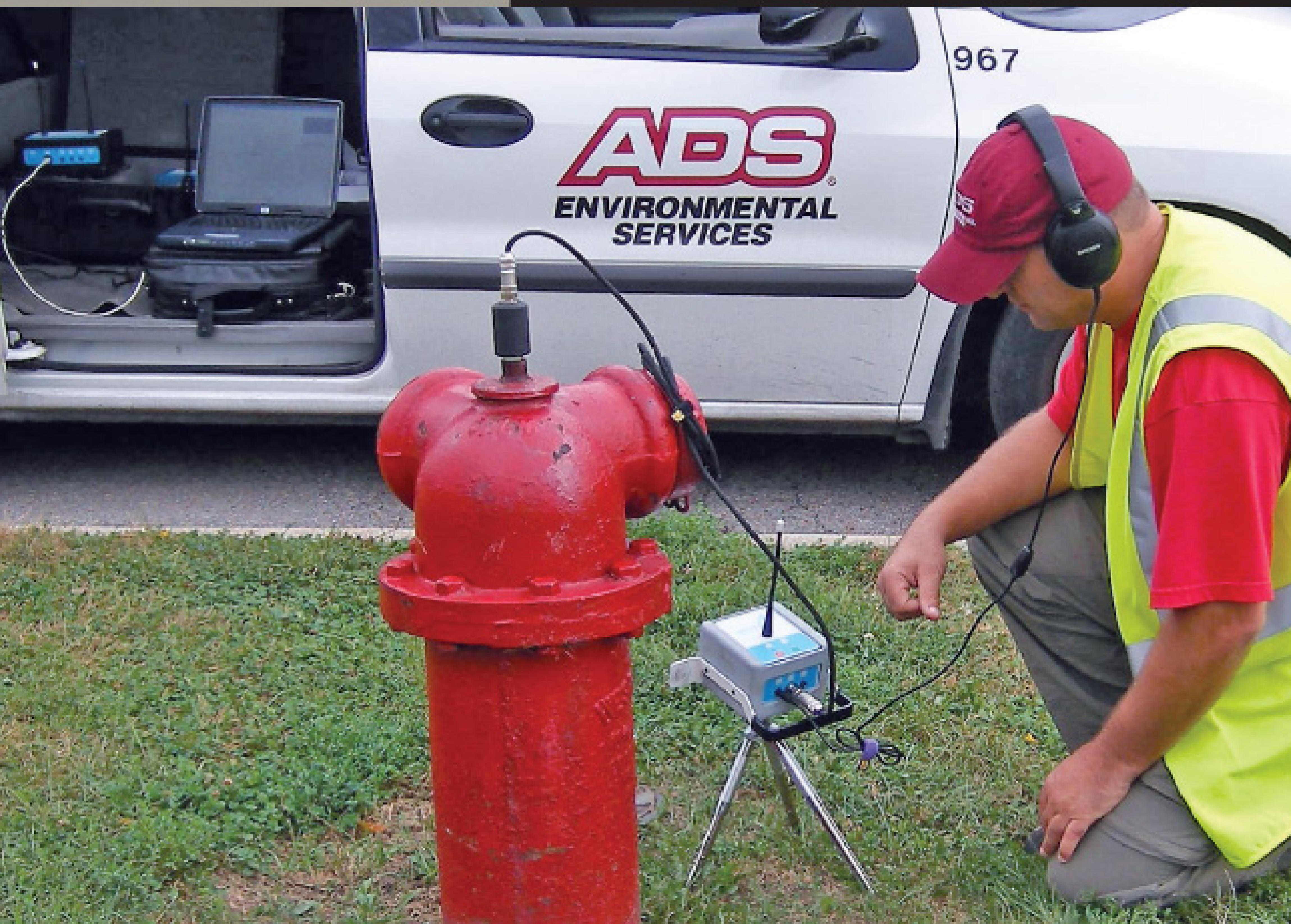
A technician with ADS Environmental Services uses the large-pipe leak correlator.
