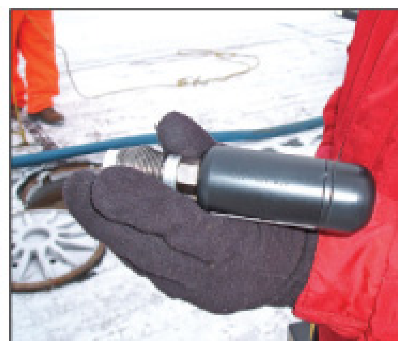
A sonde accompanies the TraceMaster II unit for locating sewer pipes.
