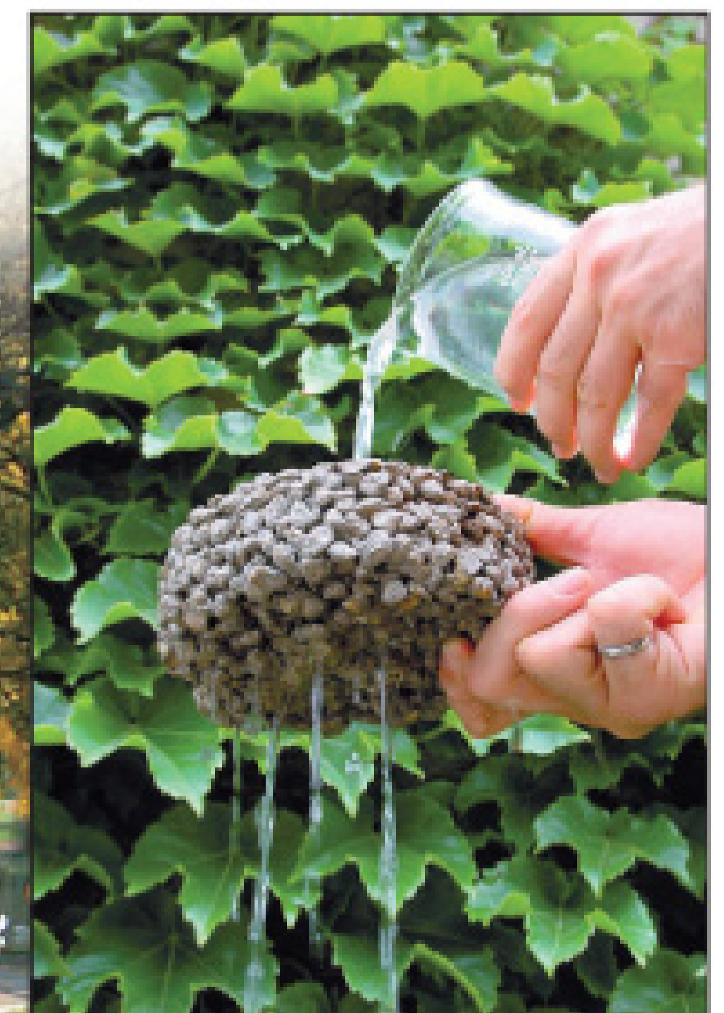
Permeable concrete pavement allows stormwater to pass directly through.
