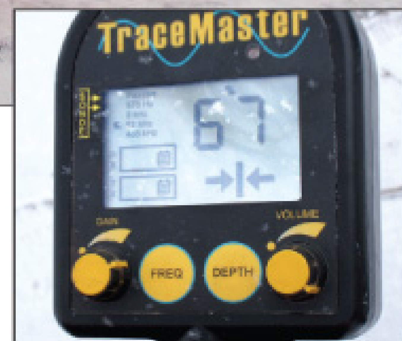
At right, the digital readout on TraceMaster II shows two arrows are pointing toward each other with a vertical bar between. This indicates that the receiver is directly over the water pipe carrying the signal from the transmitter.
