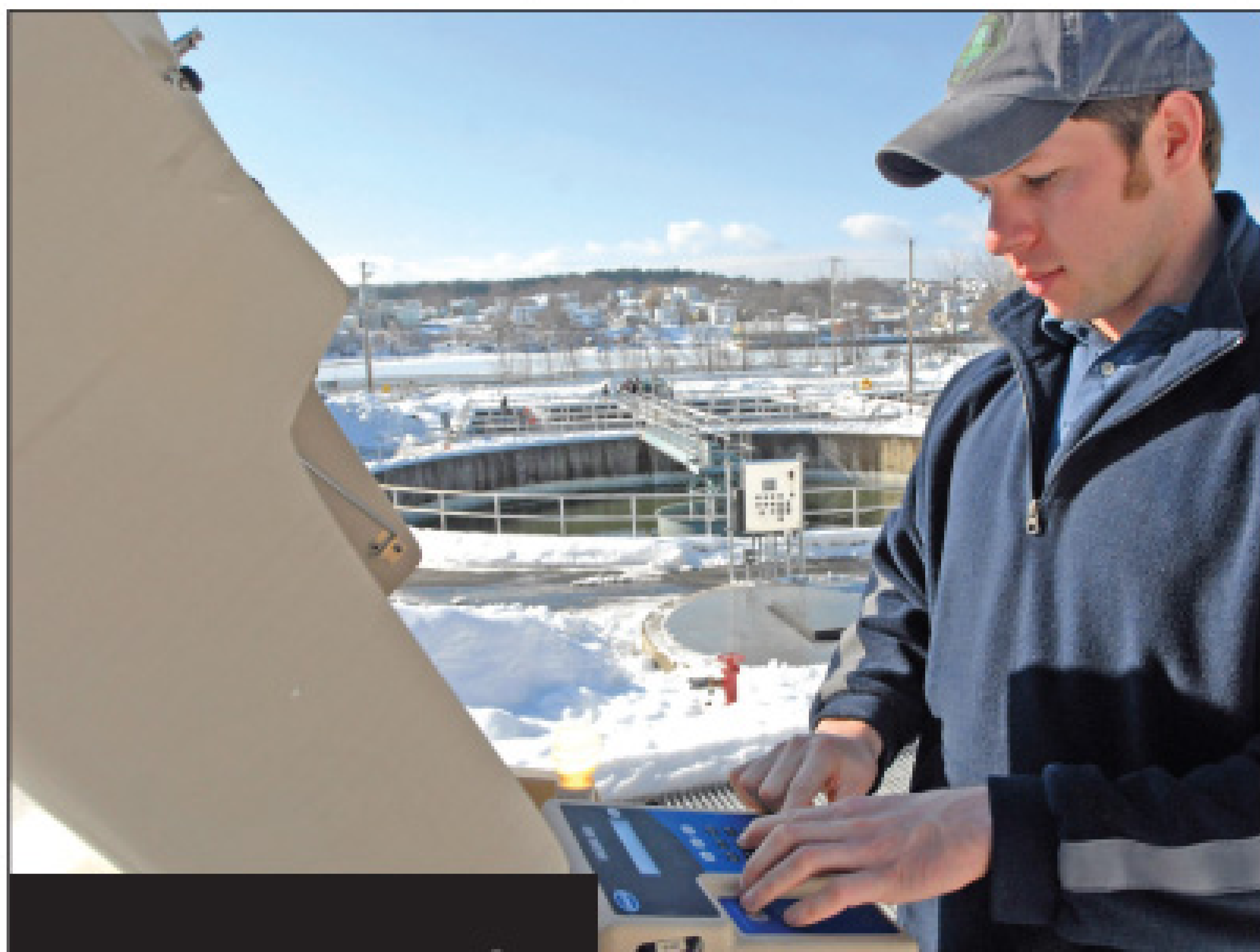
Lab technician Travis Peaslee checks the influent composite sampler at Saco's wastewater treatment plant. (Photos by Shawn Patrick Ouellette)
