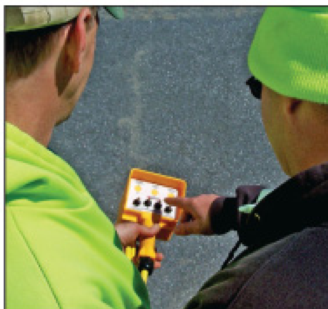
Operator Amos King (left) and water transmission and distribution supervisor Don Kirchner review the crane's tethered control system.
