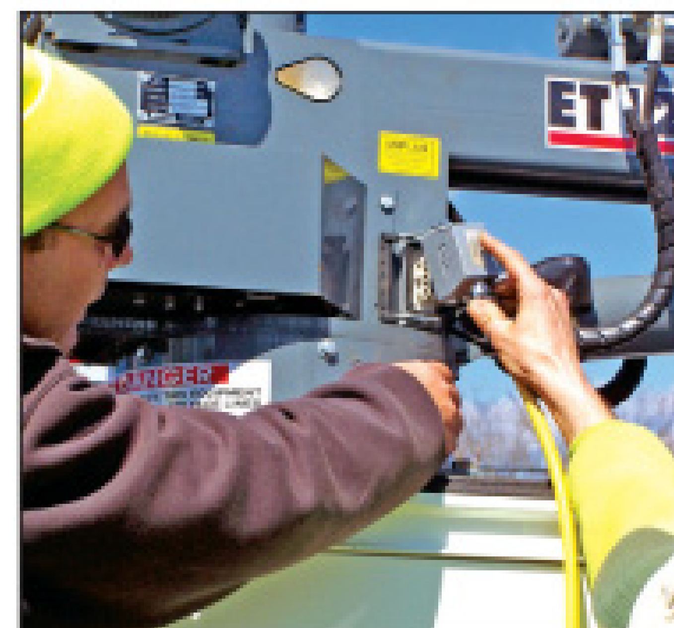
Don Kirchner (left) and King insert the crane control cable in preparation for a lift.
