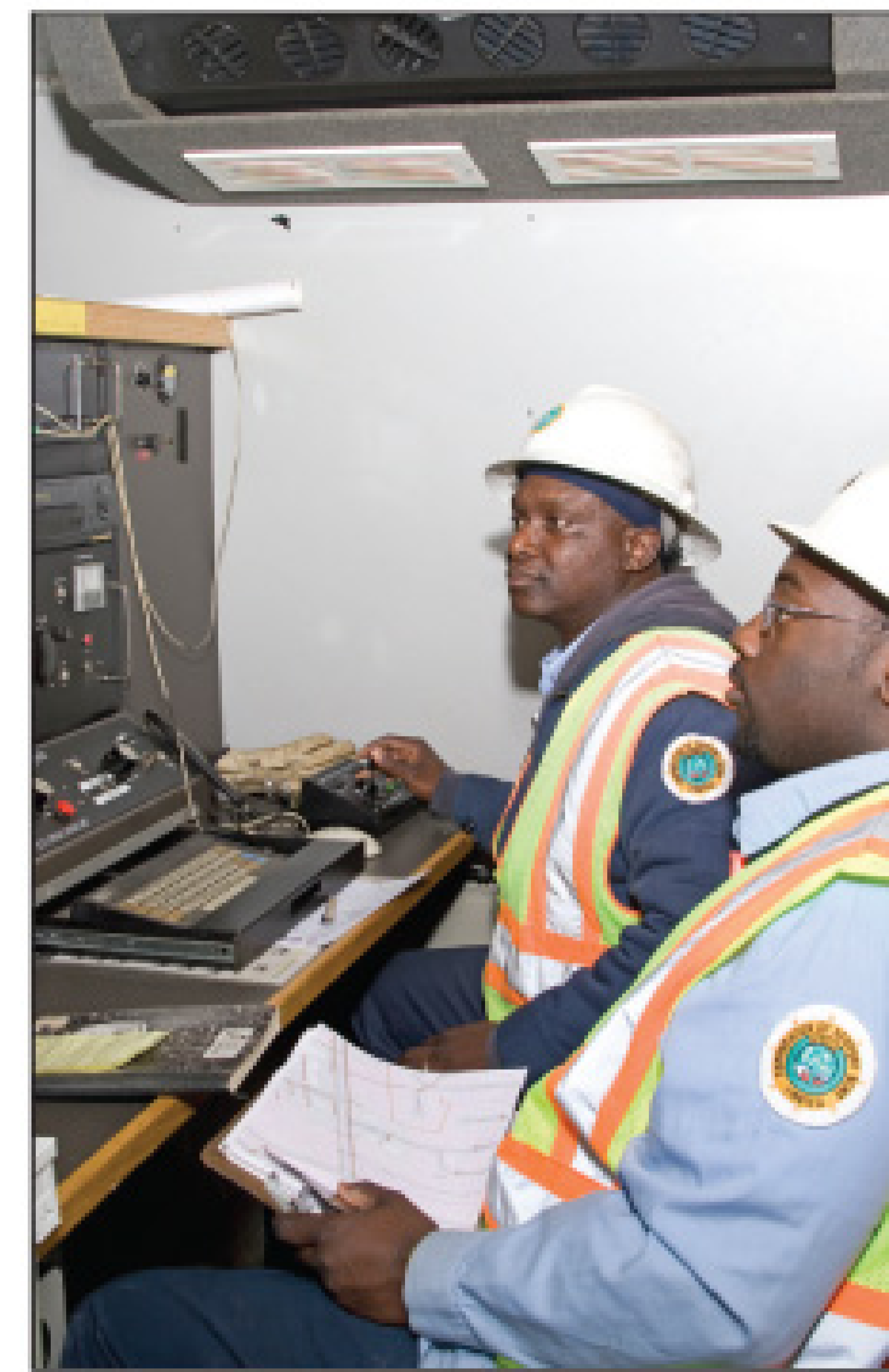
Stormwater coordinator Curtis Hartsfield (front) and Eugene Whitaker conduct a CCTV inspection of a storm sewer.
