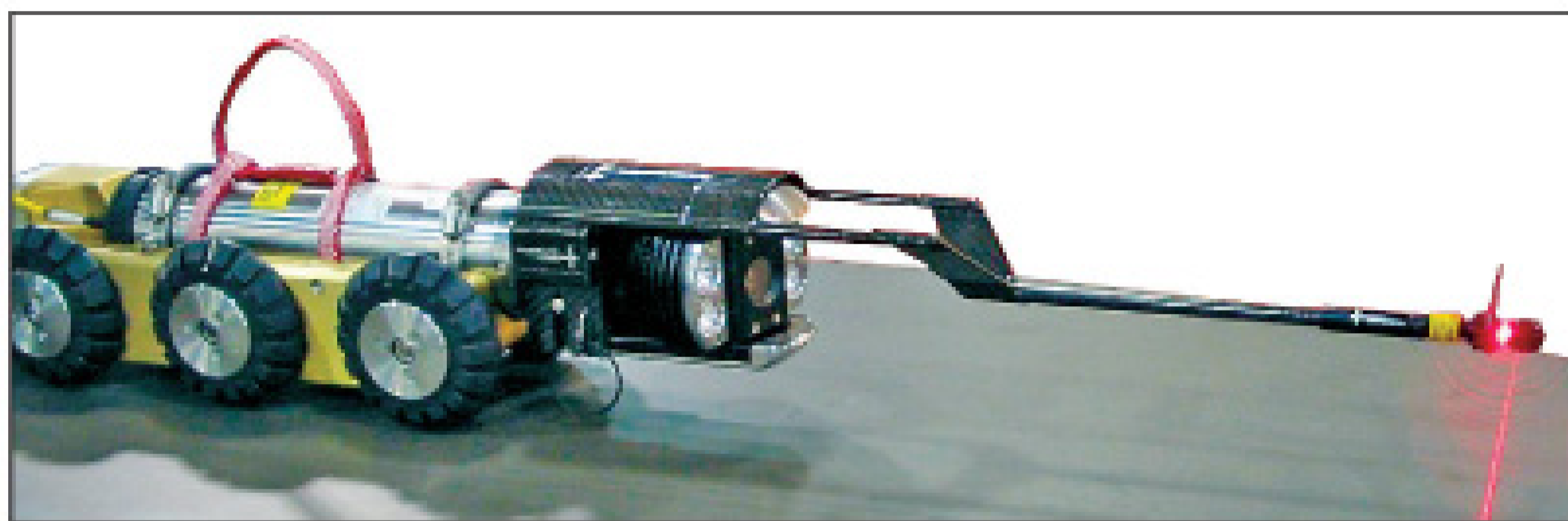
In this common laser profiling configuration, a CUES LP917 laser profiler is shown coupled with an OZII video camera.
