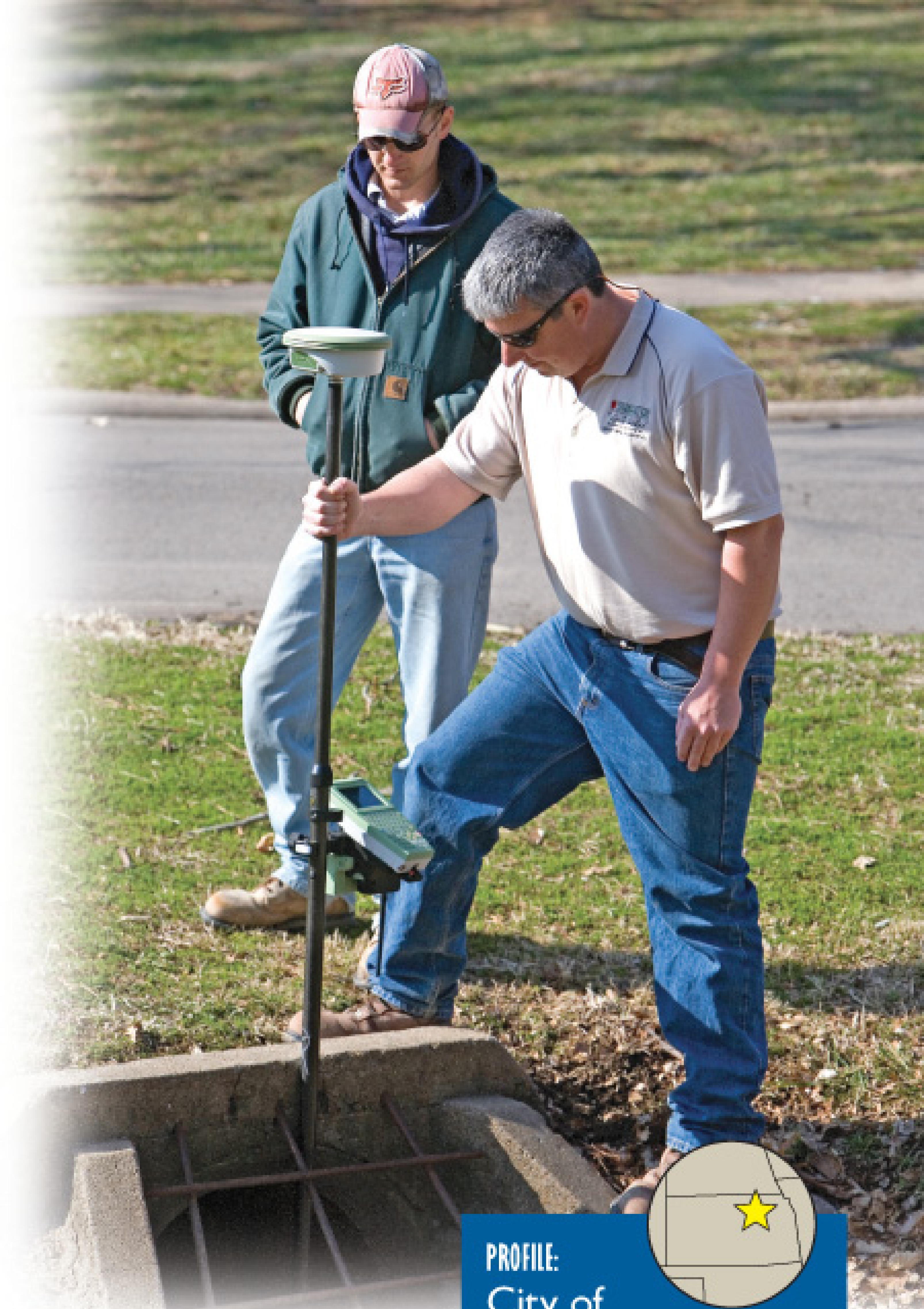
City of Manhattan crew members Ken Hays (holding rod) and Tyler McCann record the location of a stormwater inlet using a Leica 1200 GPS. (Photography by Rod Mikinski)
