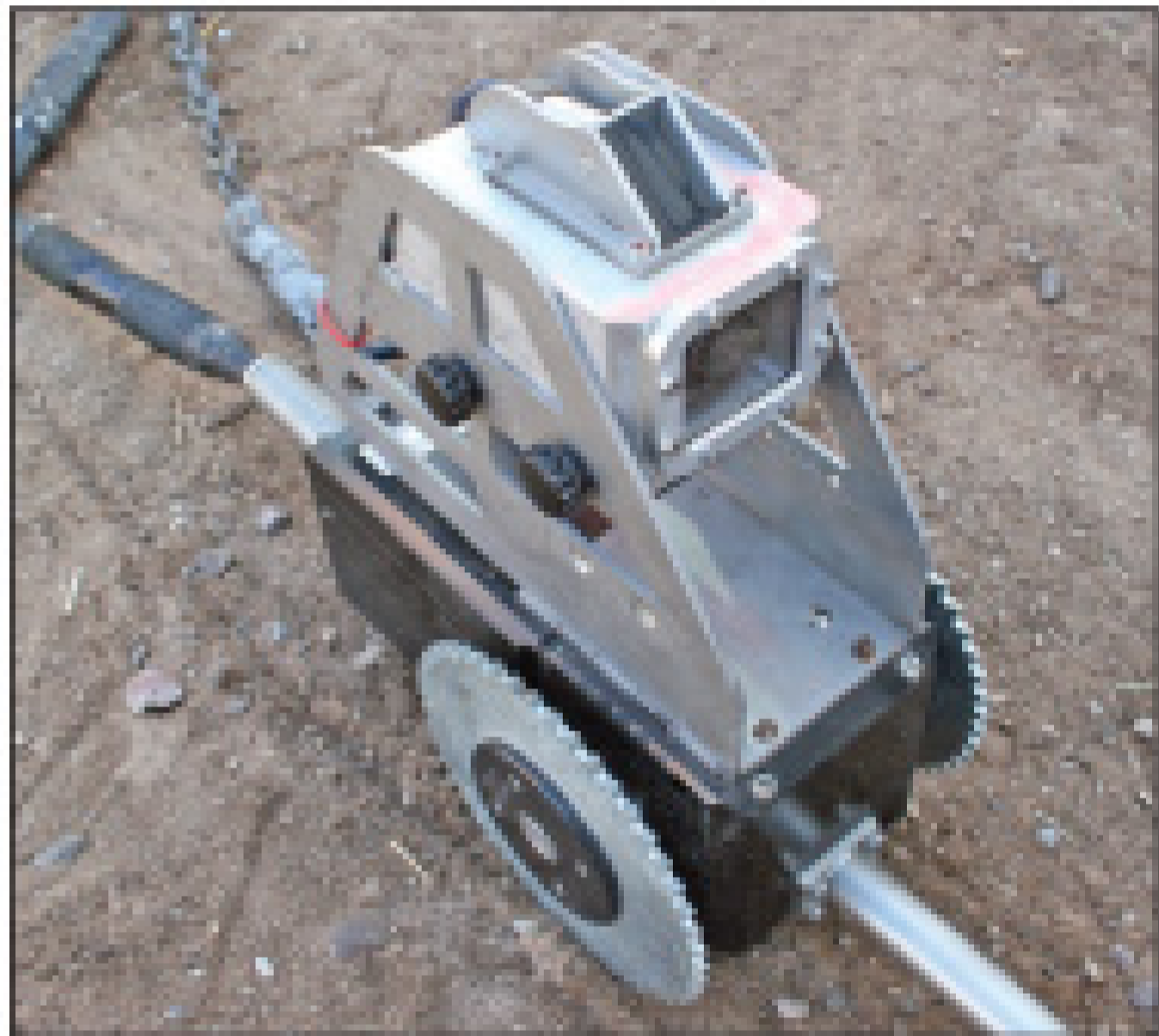
The camera module at the rear of the unit is ruggedly built and fixed in position relative to the laser module by a rigid conduit "backbone" joining the two.
