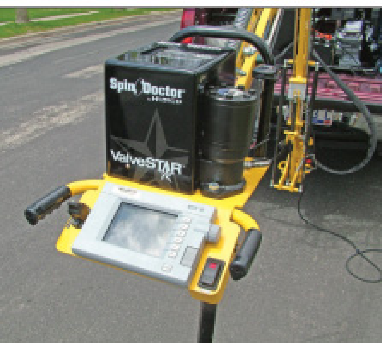
The demonstration unit includes the Valve Star head with screen for recording valve data. (Photos by Ted J. Rulseh )
