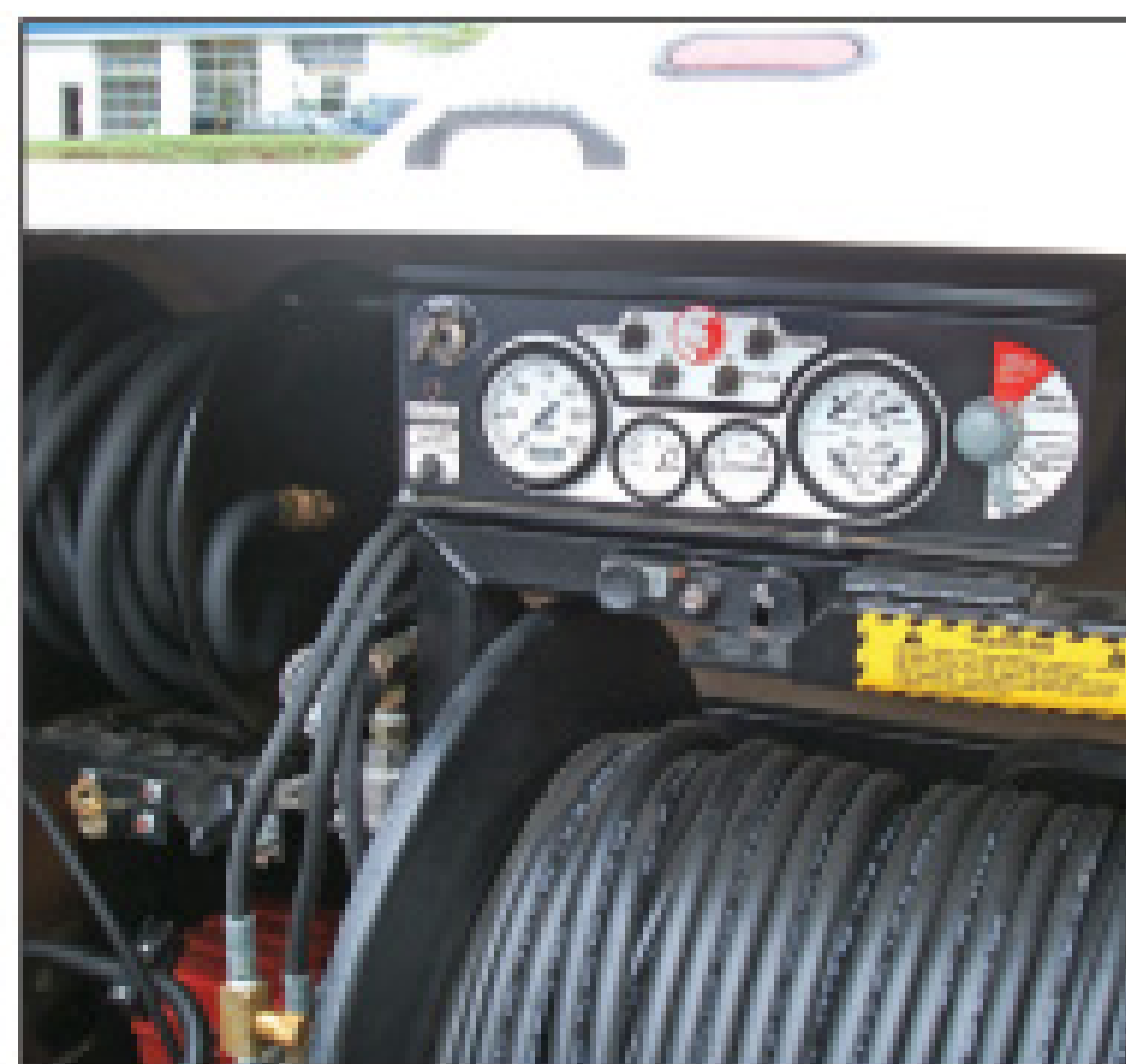
The instrument panel is located in the rear cabinet of the jetter.
