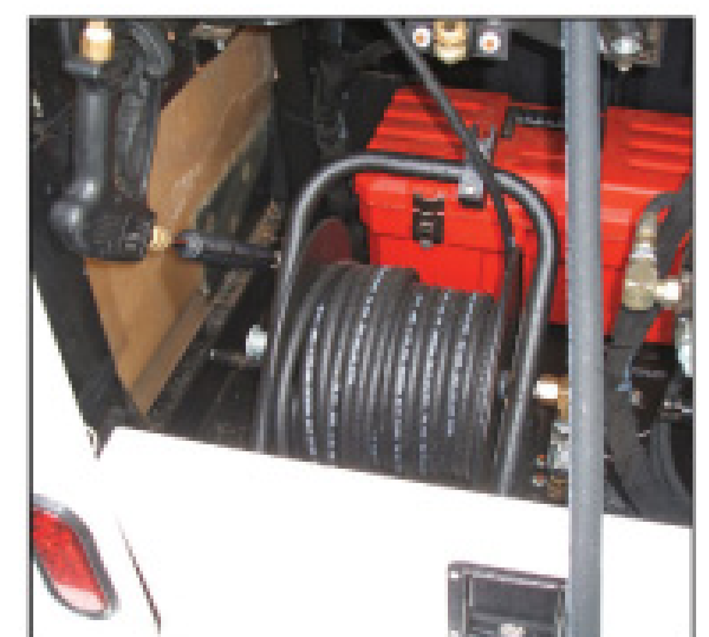
Upper right: The cleaning nozzle attached to the second jetting/wash-down hose. Lower right, the hose used for the wash-down nozzle or to jet in more limited spaces.
