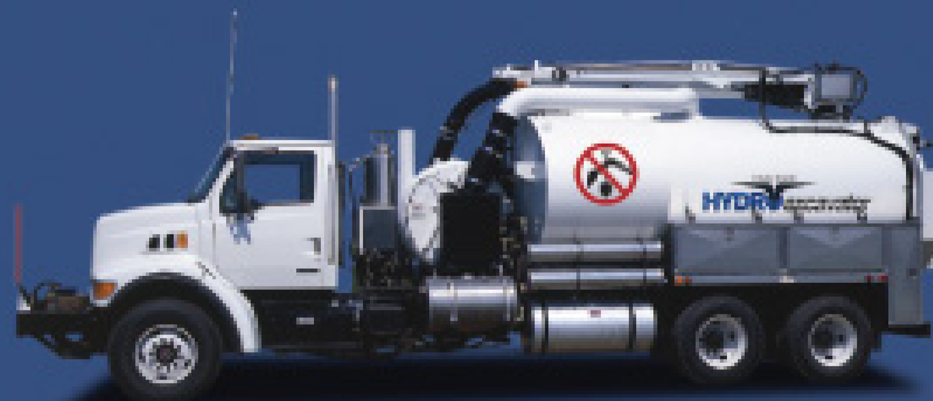
HXX Full-sized HydroExcavator Breaks soil apart with pressurized water Excellent for big digs and deep trenching
