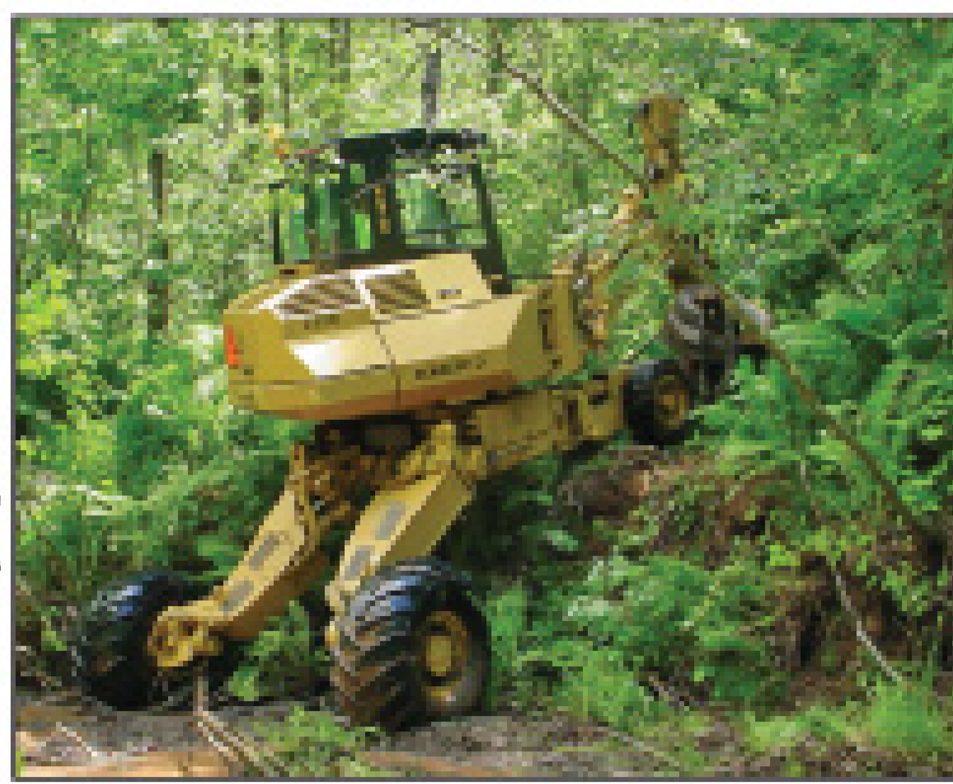
The telescoping legs of the HS 41 Spider by the Schaeff Co. make it ideal for working in uneven terrain.
