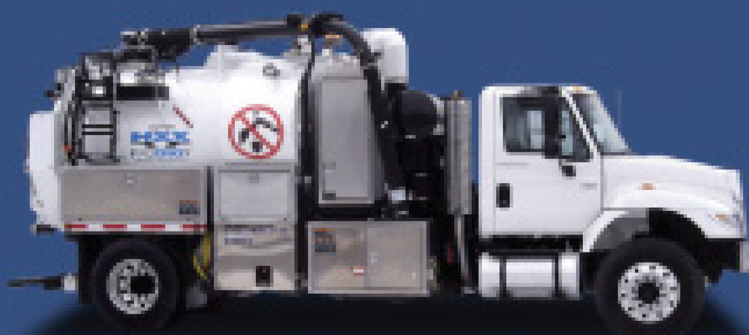
HXX Prodigy Mid-sized Vacuum Excavator Excavates with water or optional air Perfect for potholing or locating
