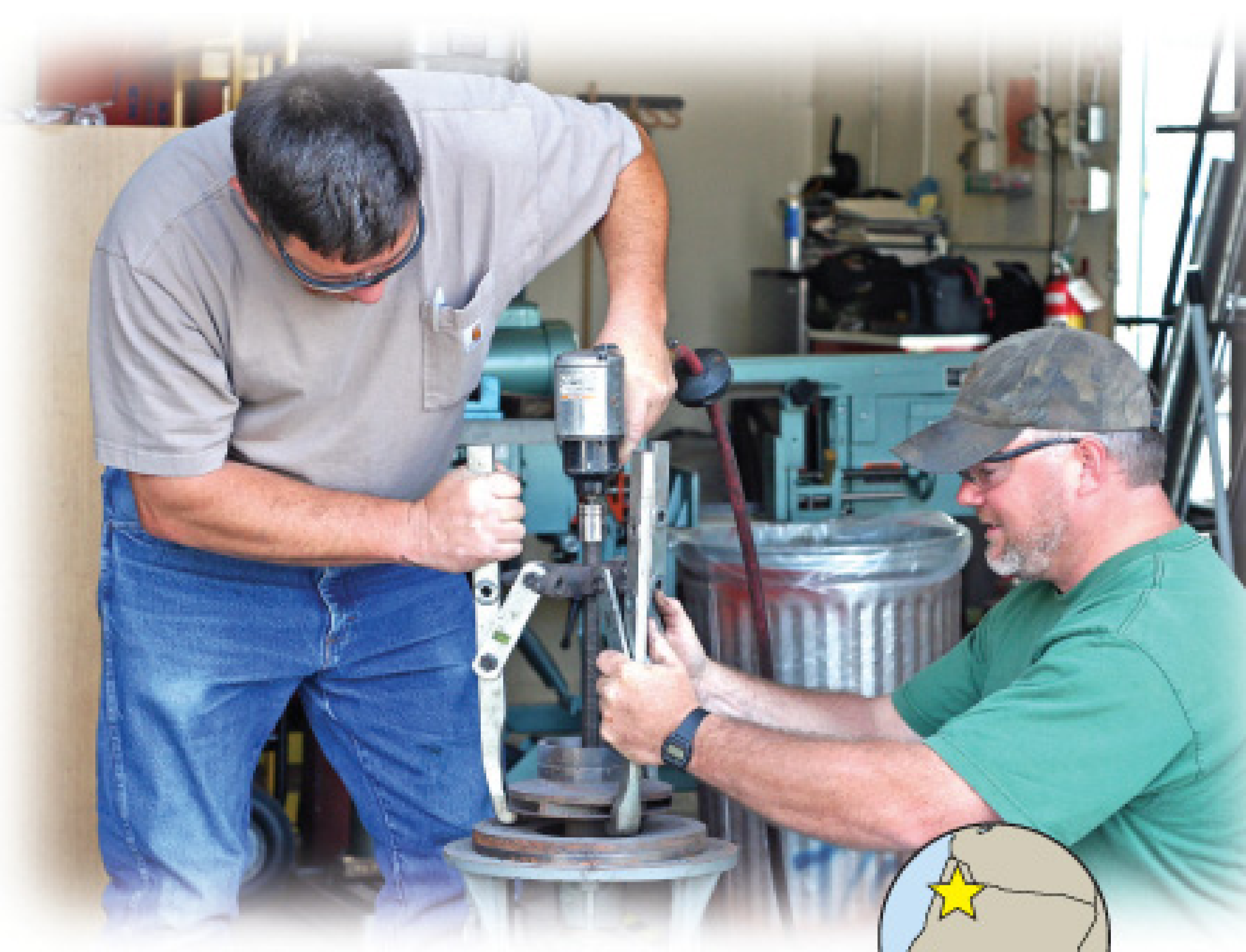
Gerald Arredondo (left) and Shane Wallen of the Salem Pumps and Controls Group pull an impeller off of a water pump. When plugged impellers on sewage pumps at some locations required almost daily repairs, the Salem team decided to try a new style of pump that's more efficient — dry pit submersible pumps from ITT Flygt Corp. (Photography by Caryl Young)
