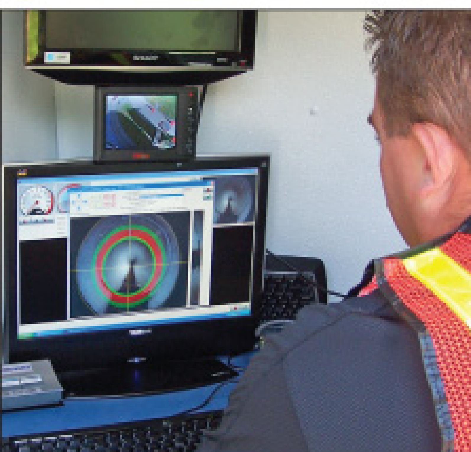
Digital images acquired by the camera are easily analyzed on a computer screen. In this case, ScanExplorer from WinCan America Inc. is used. The software provides four views: straight ahead, side view, 3-D and thumbnail. Users can zoom in on areas of interest and make measurements and annotations directly on the scan.
