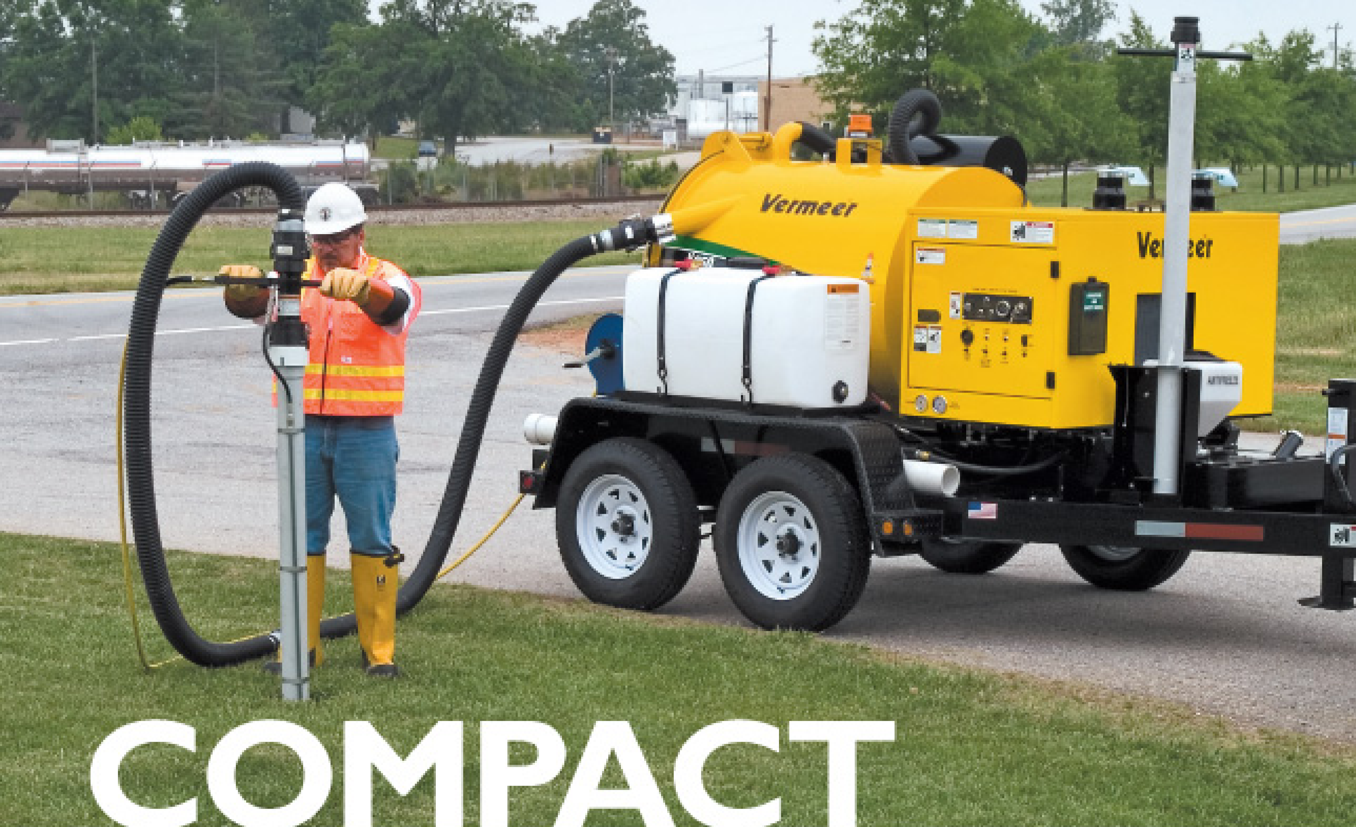
The V250 hydro vacuum excavation system from Vermeer offers contractors and municipalities a low-cost, portable system for potholing and vacuum applications.
