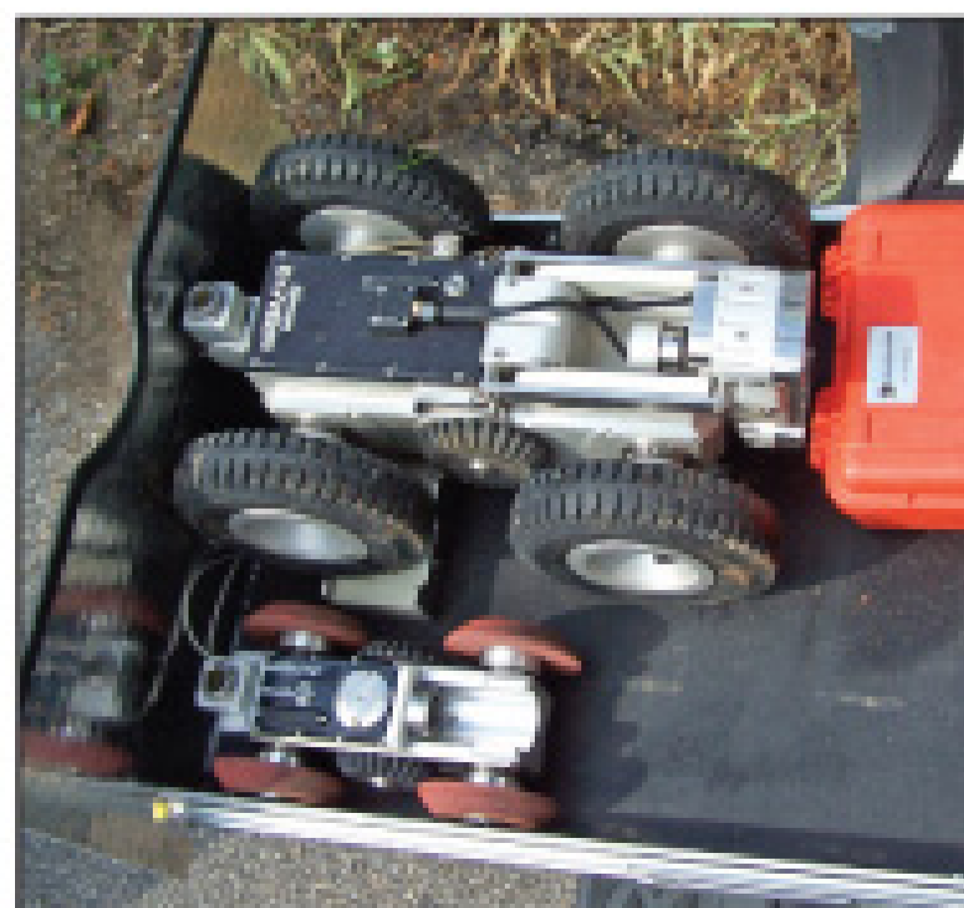
The DigiSewer system is designed to work with ROVER crawlers from EnviroSight LLC.
