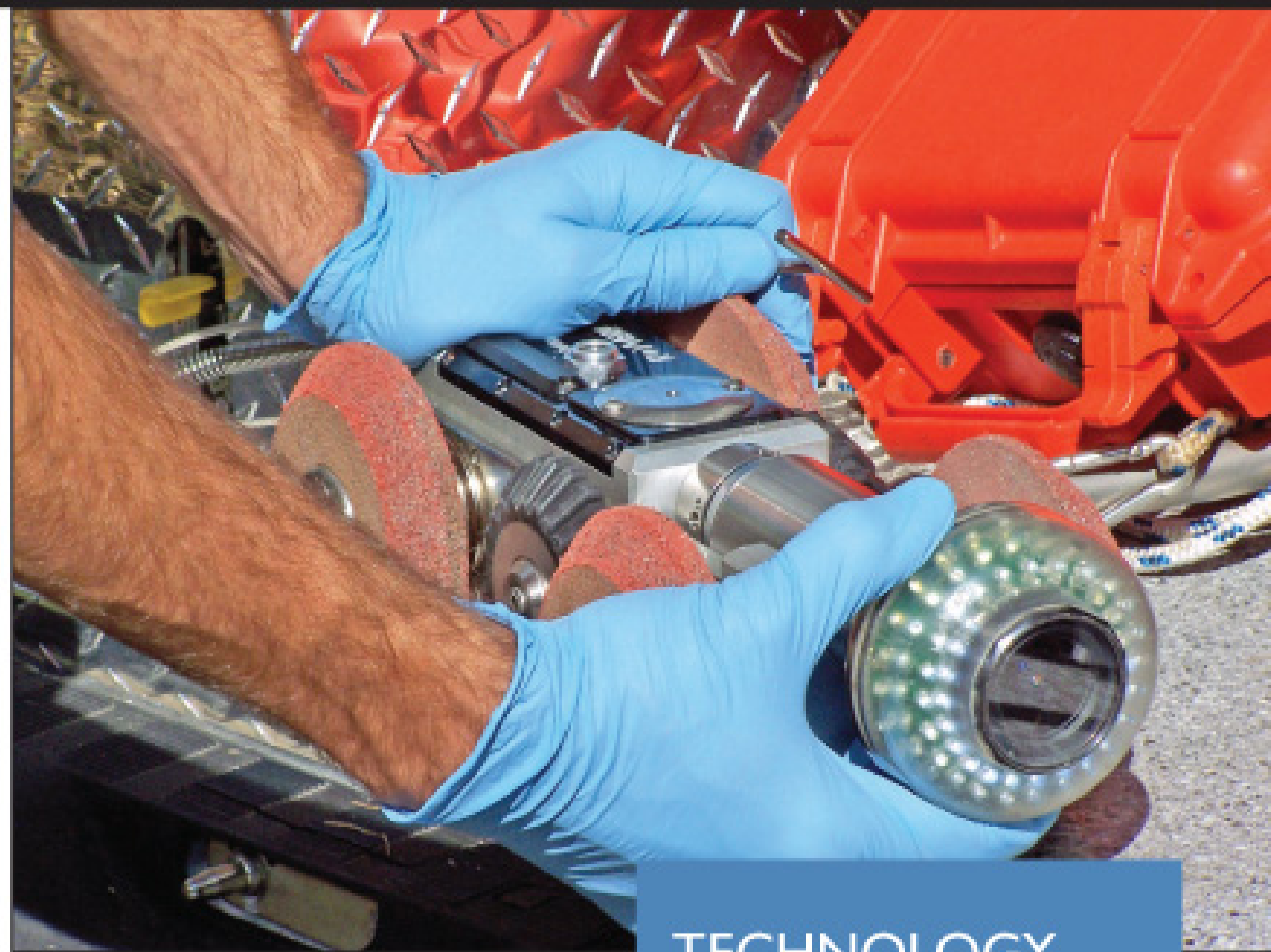
The DigiSewer 180° Inspection System rapidly acquires sidewall scan images of pipes for later review and reporting.
