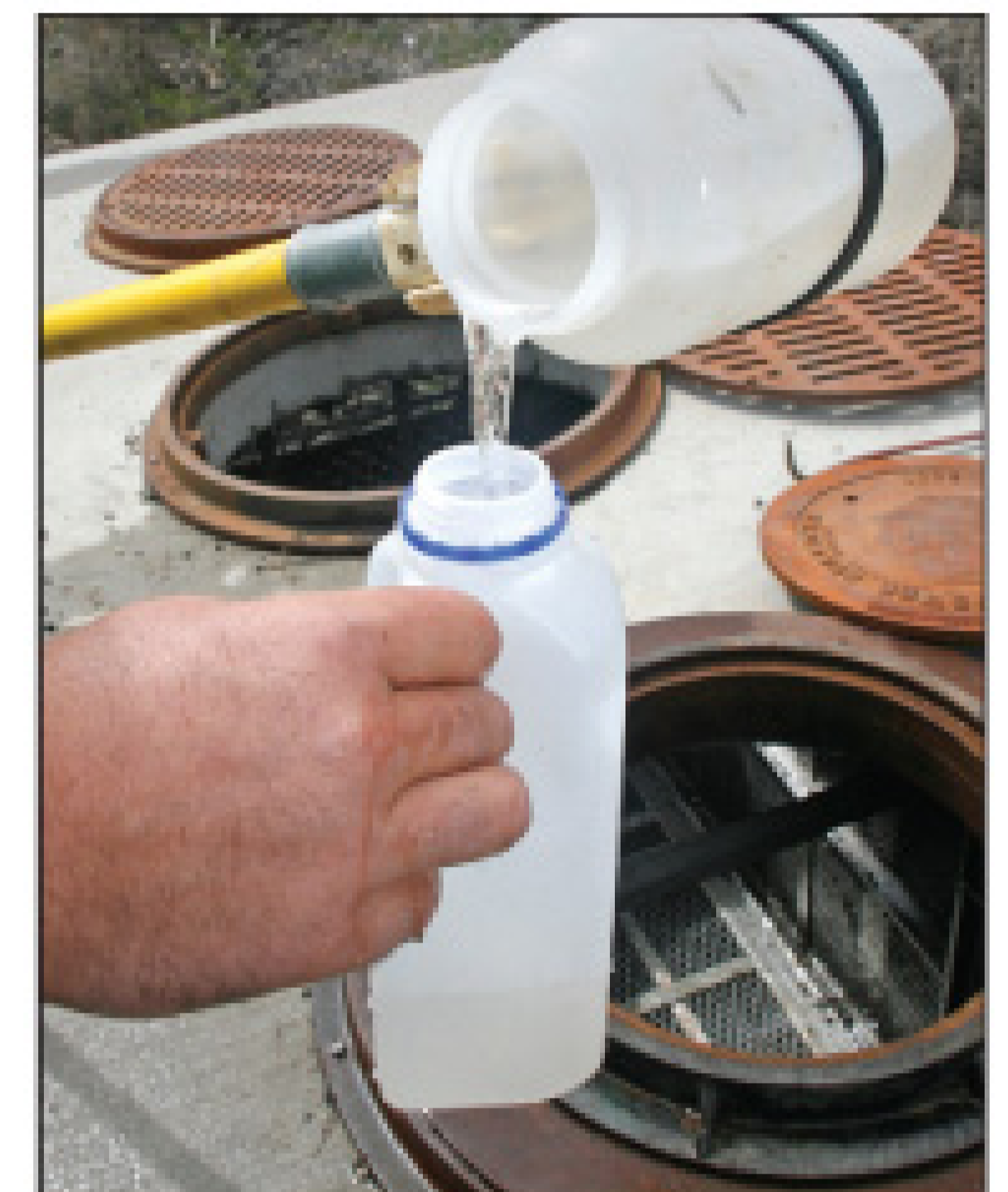
Water samples from a stormwater containment water-quality vault to check vault efficiency.
