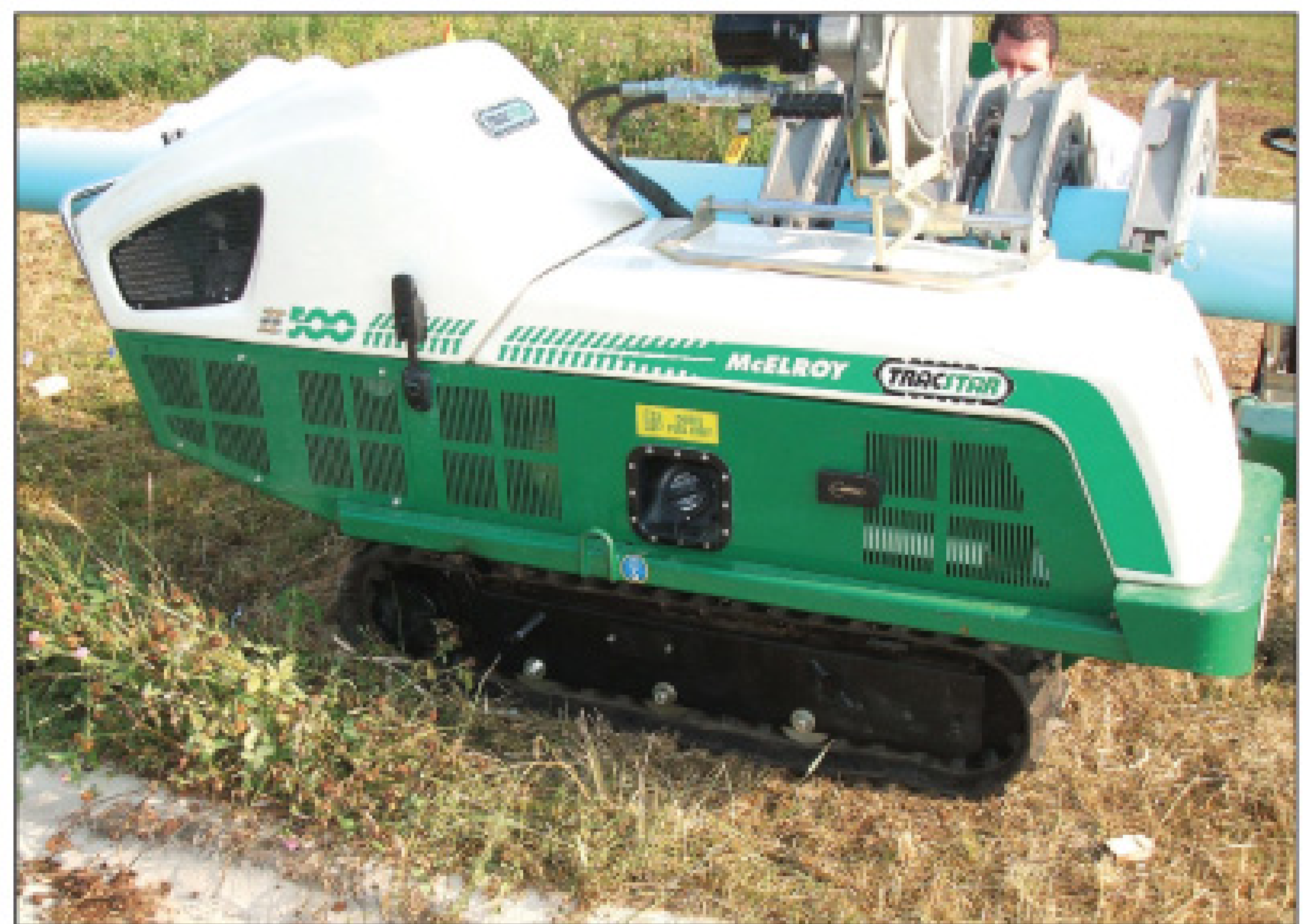
Above: The McElroy TracStar II 500 unit was used for fusing the PVC pipe sections. Right: A heated disk is placed between the ends of two lengths of pipe to be fused. The heat causes the ends to flare.
