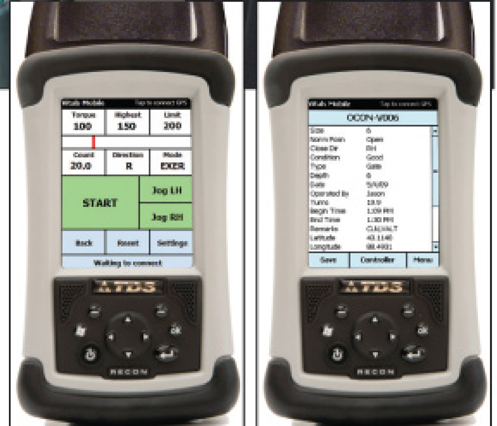
Left photo: The control module display indicates turns and torque as the system operates the valve exerciser. Users press the start button and watch as torque and direction are controlled automatically. Right photo: Users can quickly view the attributes for valves and edit as needed. Field names and drop-down lists can be customized.
