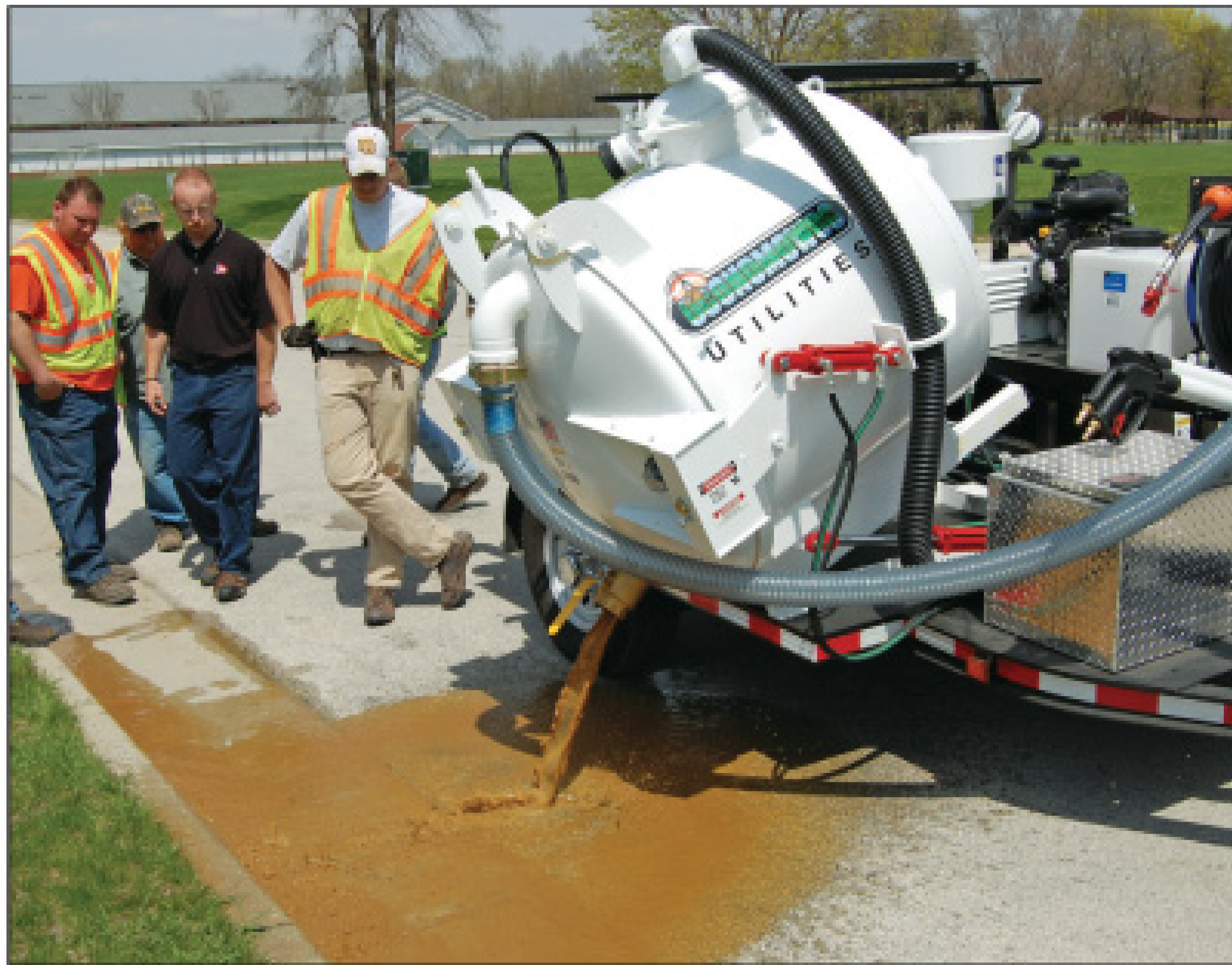
A hydraulically driven system extends the debris tank from the trailer and tilts it for dumping. (Controls for this function are on the opposite side of the trailer.)
