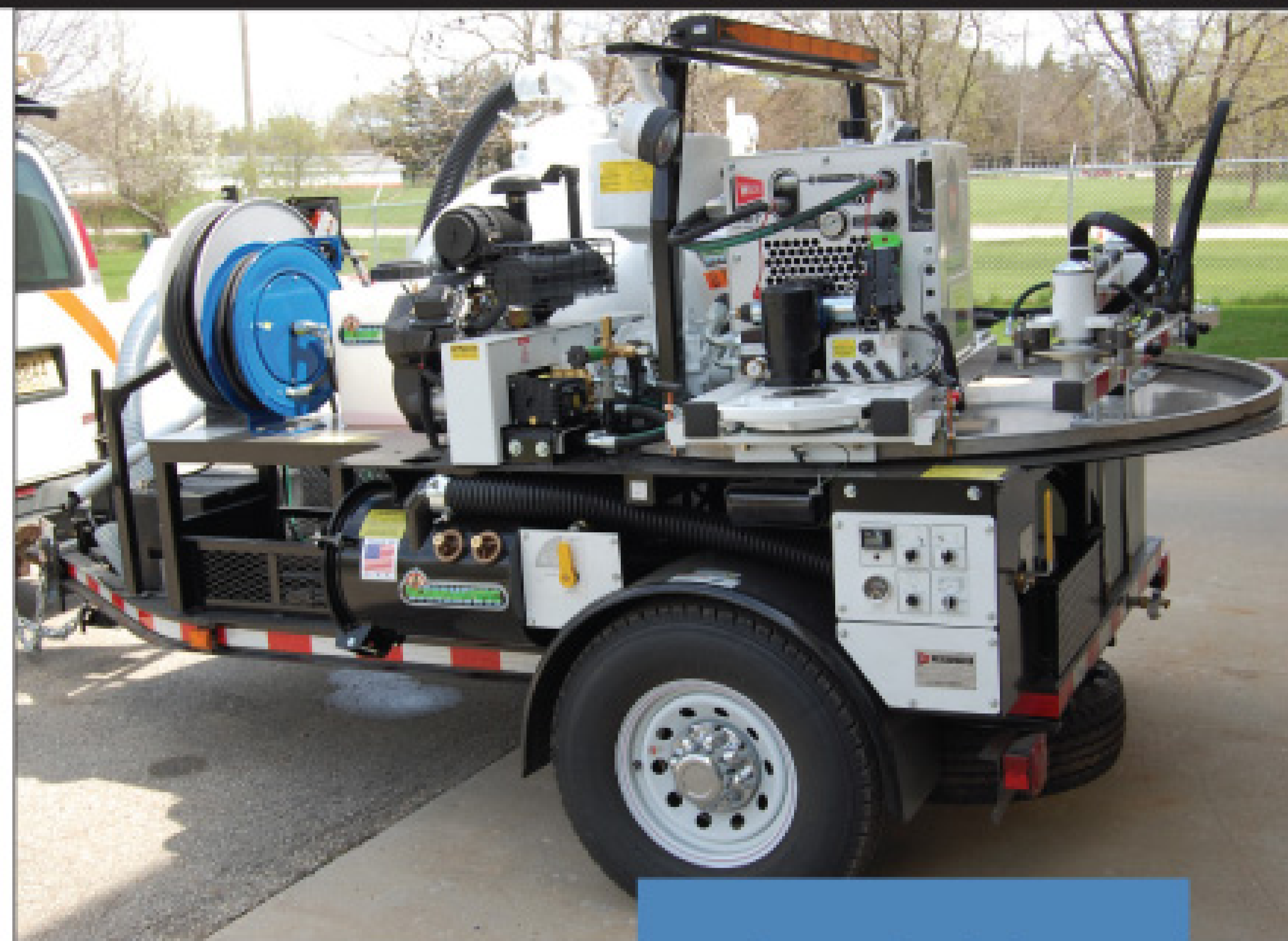
The City of Oconomowoc's VMT-1 valve maintenance trailer from E.H. Wachs Co. includes the ERV-750 extended-reach exerciser and the TM-7 heavy-duty exerciser. (Photography by Ted J. Rulseh)
