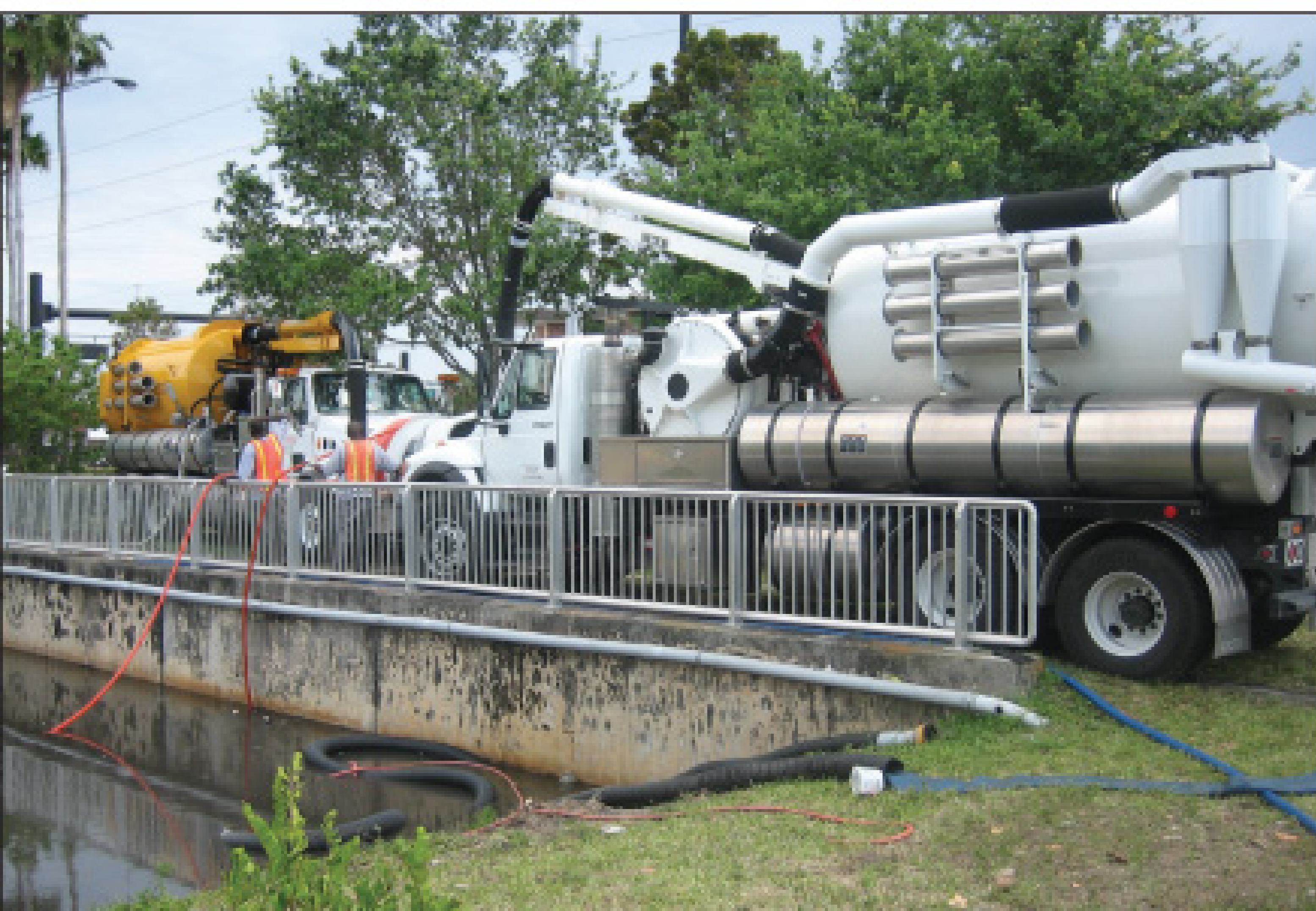
Vincent Farquharson (left) and Roscoe Graham supervise the feeding of the hose. The Vactor 2100 combination truck is on the left, and the Vactor 2100 Plus fan-driven vacuum truck is on the right.
