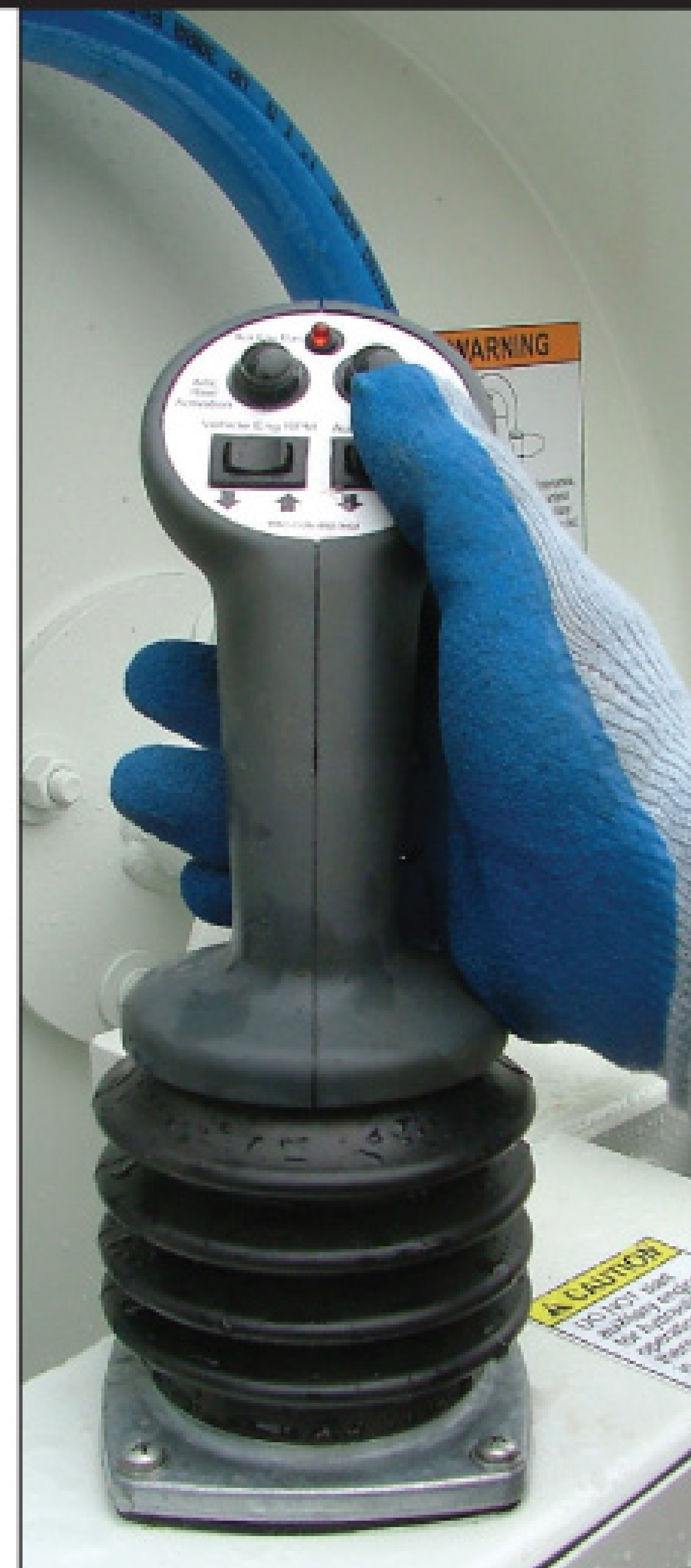
The Omnibus controller for Vac-Con combination trucks and hydroexcavators lets operators control all basic water and vacuum system functions with one hand. (Photos by Jim Force)
