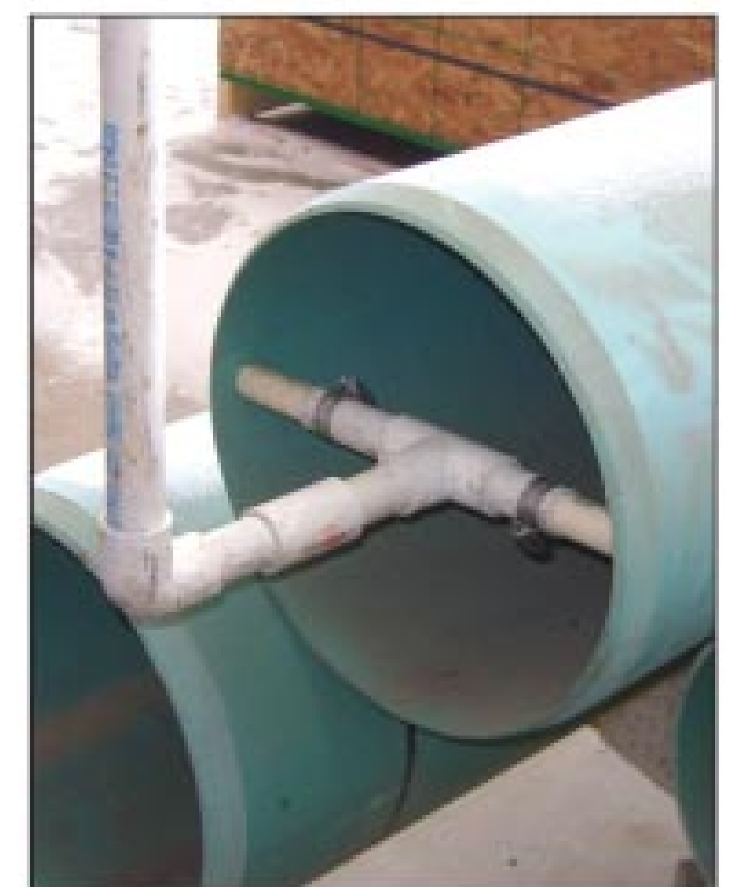
The tool helps sewer workers differentiate between pipe sizes without having to enter a manhole. It can be built with $10 to $15 worth of materials.
