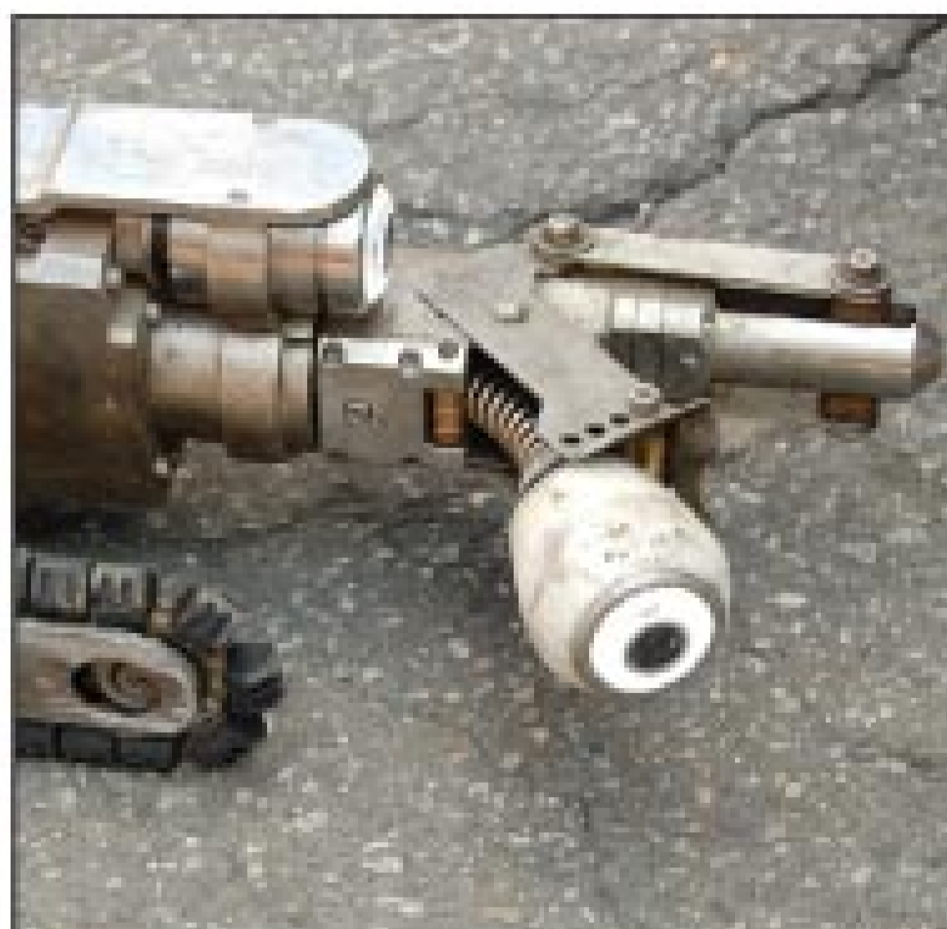
A movable chute at the front end of the inspection crawler enables the camera head to tilt up and down and rotate to the side. The camera head also extends outward to travel up the lateral.
