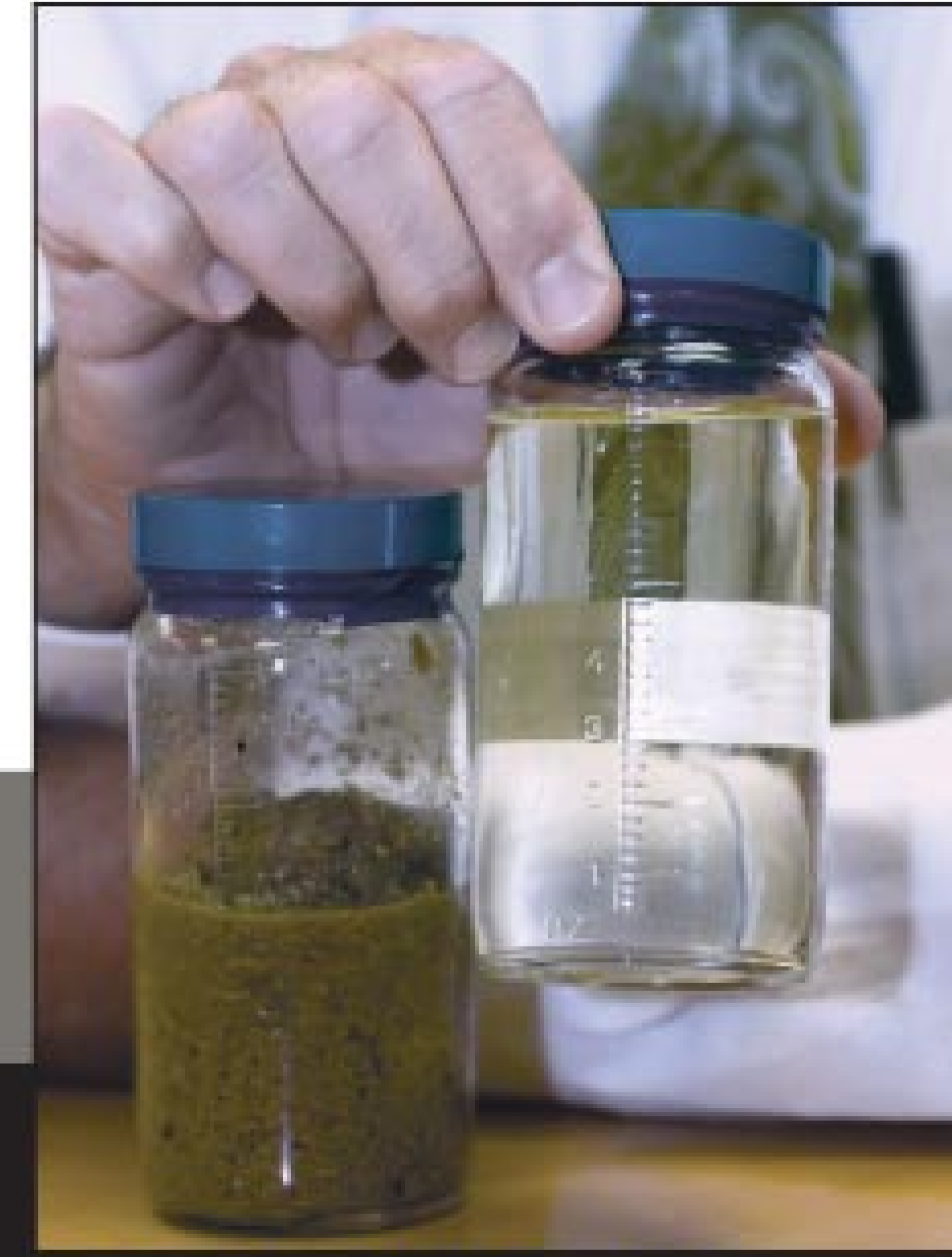
Used cooking oil before and after processing into biofuel.
