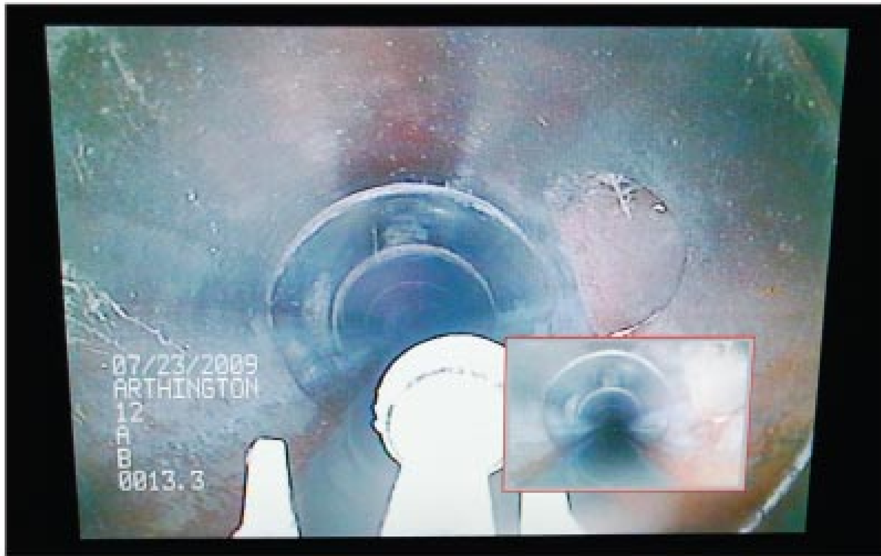
A picture-in-picture feature allows the operator to see the views from the spotter camera and lateral camera at the same time. In this image, the full-screen picture is the spotter camera's view and the inset is the lateral camera's view. Note the lateral opening at the right center of the screen. At the flip of a switch, the operator can reverse the priority so that the full-screen image is the lateral camera's view.
