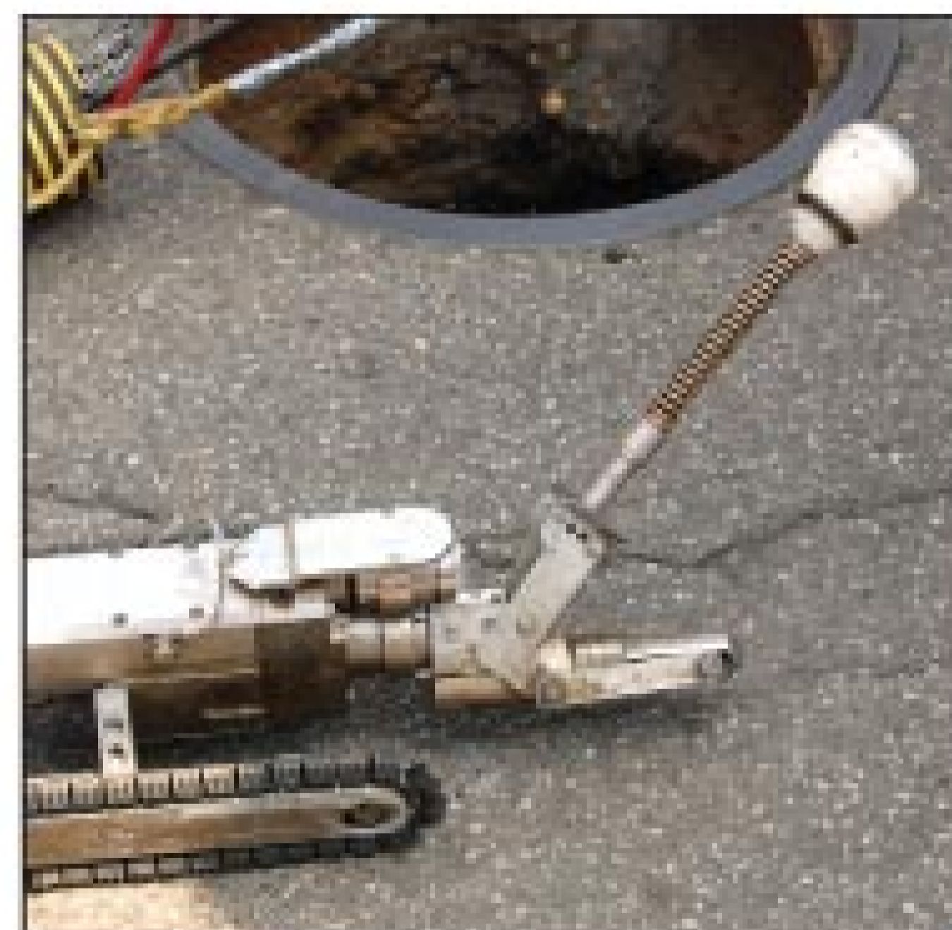
A movable chute at the front end of the inspection crawler enables the camera head to tilt up and down and rotate to the side. The camera head also extends outward to travel up the lateral.
