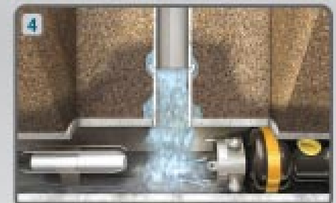
Water infiltration at lateral
