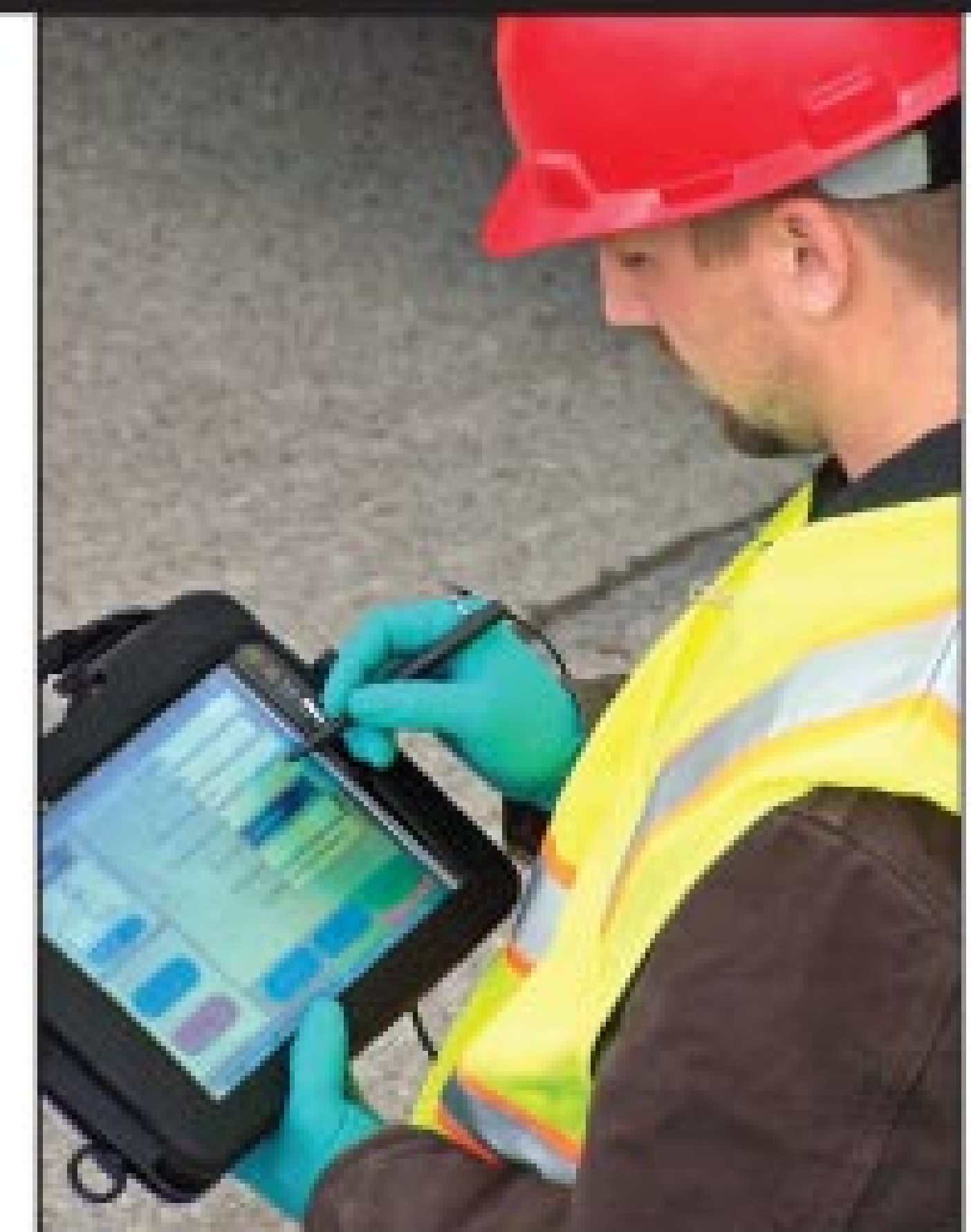
An armored tablet computer with WiFi capability transmits location and pipe information to the crawler and is used to send the unit on its way.
