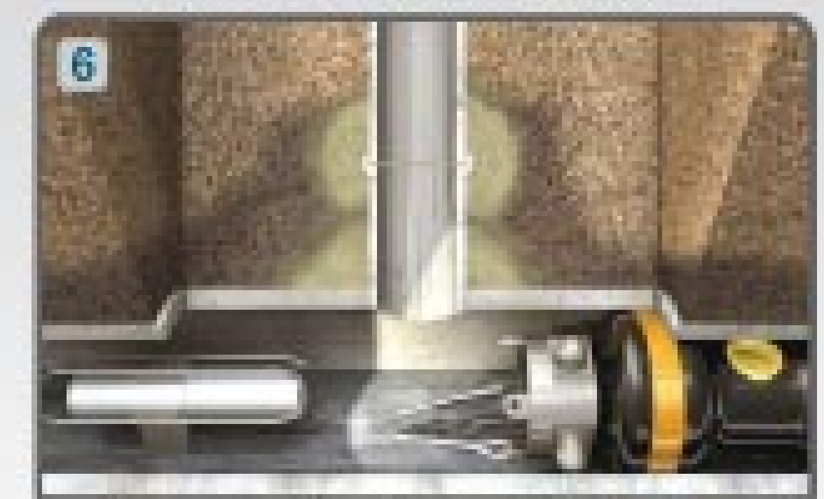
Grout collar stops infiltration
