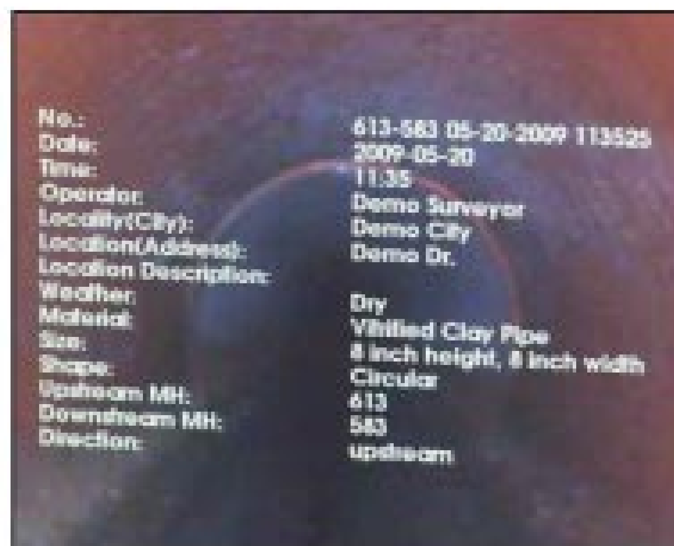
Left, a data overlay on the control screen shows basic information about the pipe being inspected. Right, an image from inside a pipe shows a plugged lateral.
