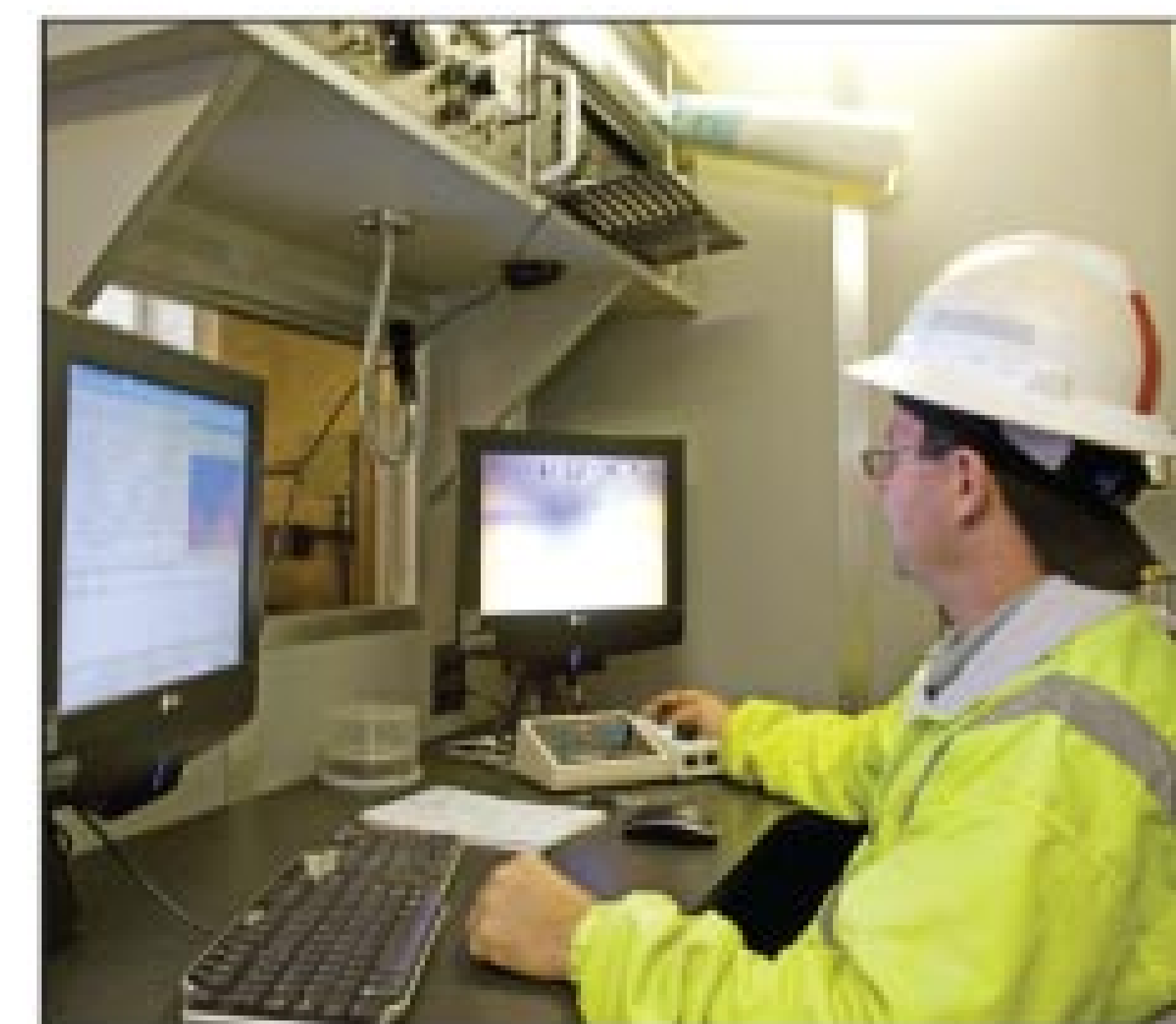
Brian Bickers observes a sewer line from an inspection van console.
