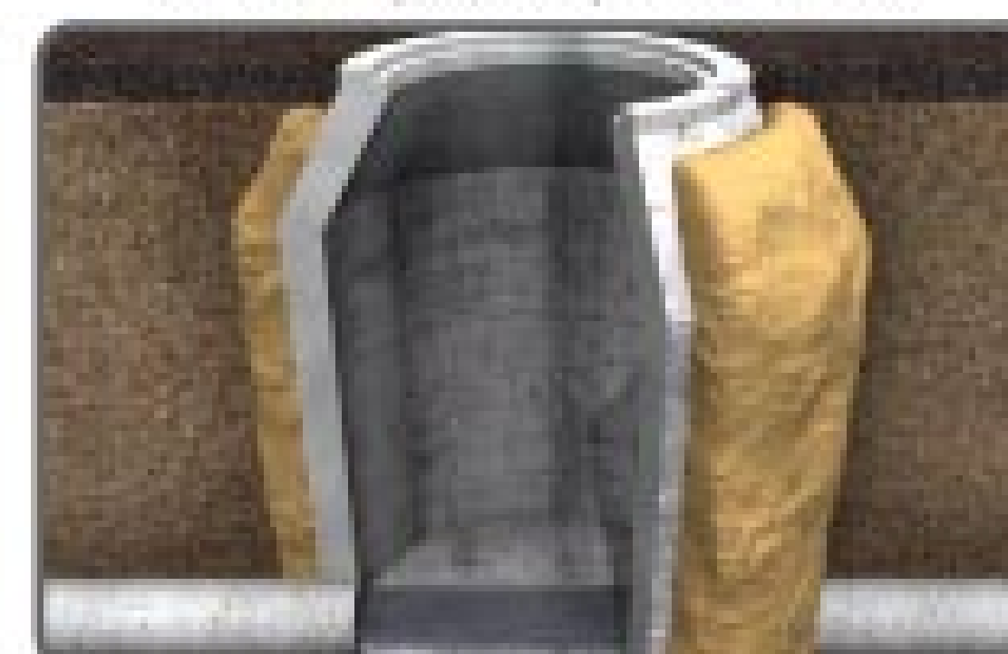
Grout curtain stops infiltration
