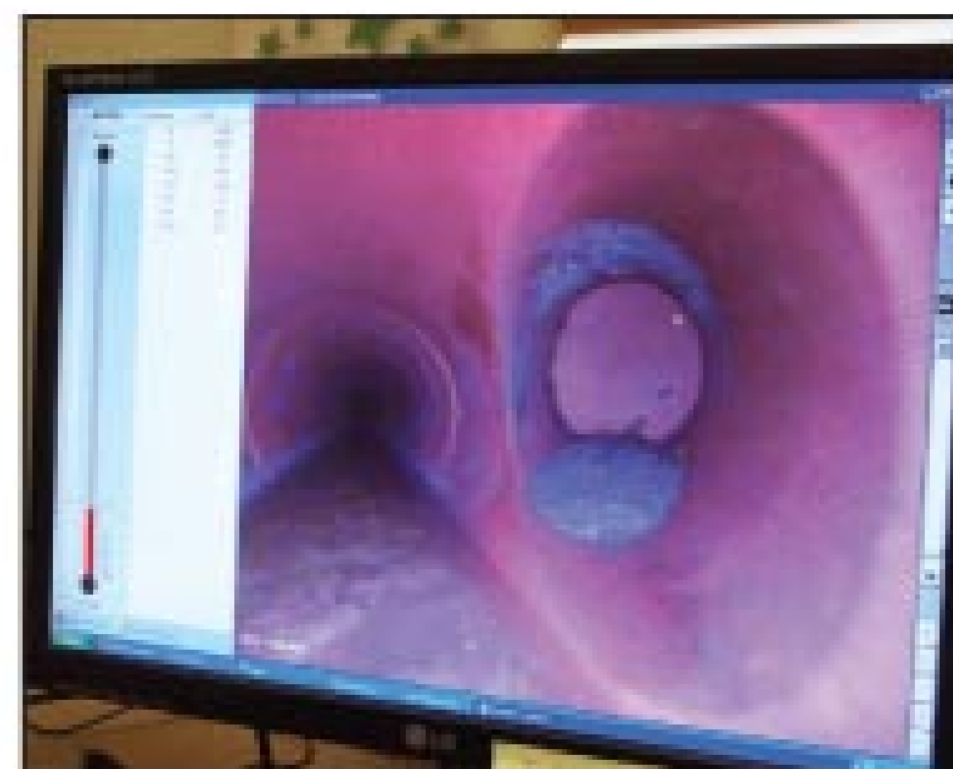
Left, a data overlay on the control screen shows basic information about the pipe being inspected. Right, an image from inside a pipe shows a plugged lateral.
