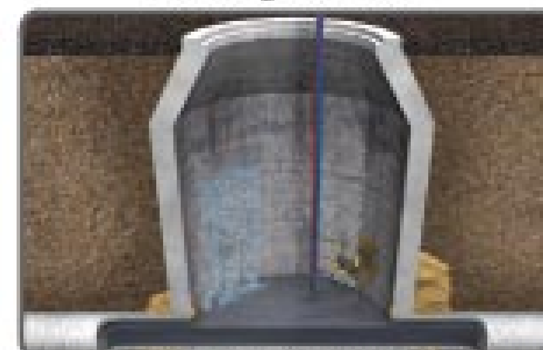
Curtain grouting with wand
