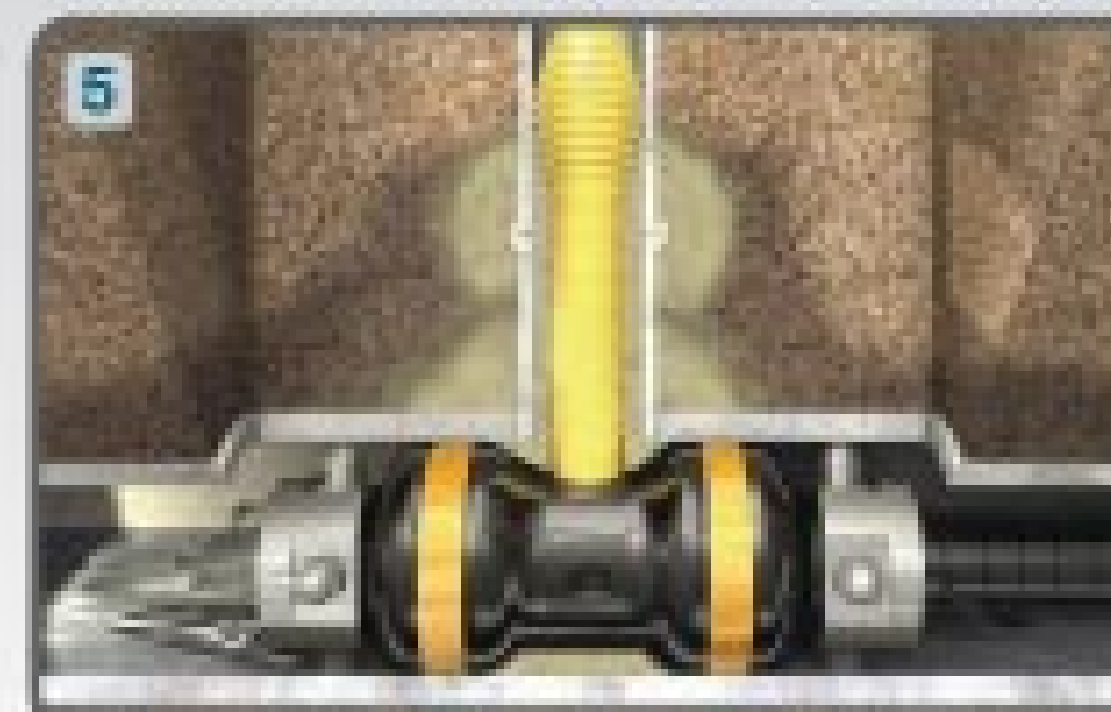
Lateral packer injecting grout
