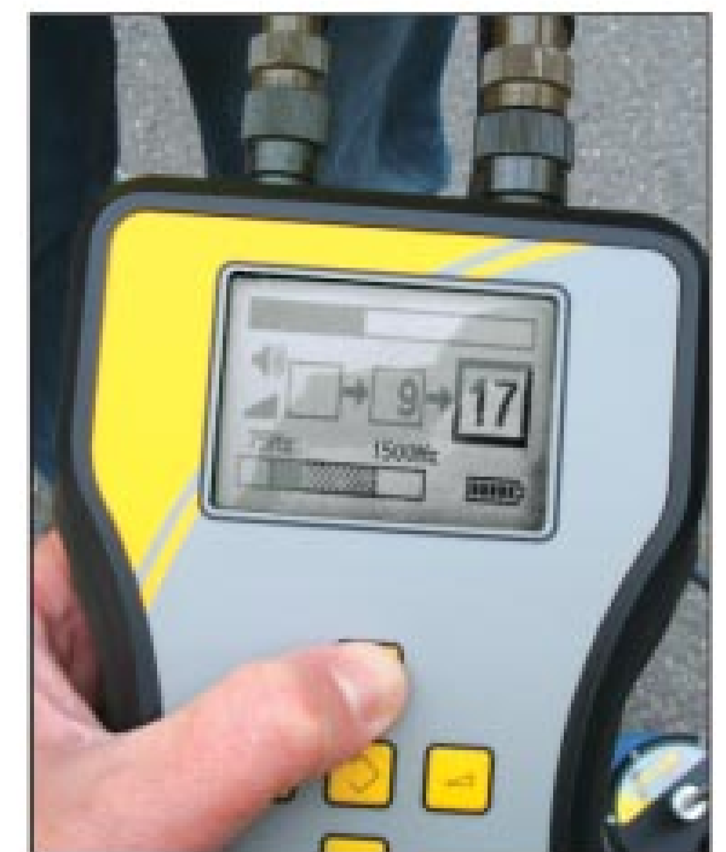
The Mikron control panel. The center box shows a number (9) that was captured at one point during the ground microphone’s use as the operator, Bill Doyle, walked it along the length of an underground pipe in search of the leak. The right box is the real-time index number, 17, at his current location, indicating he is now closer to the leak source.
