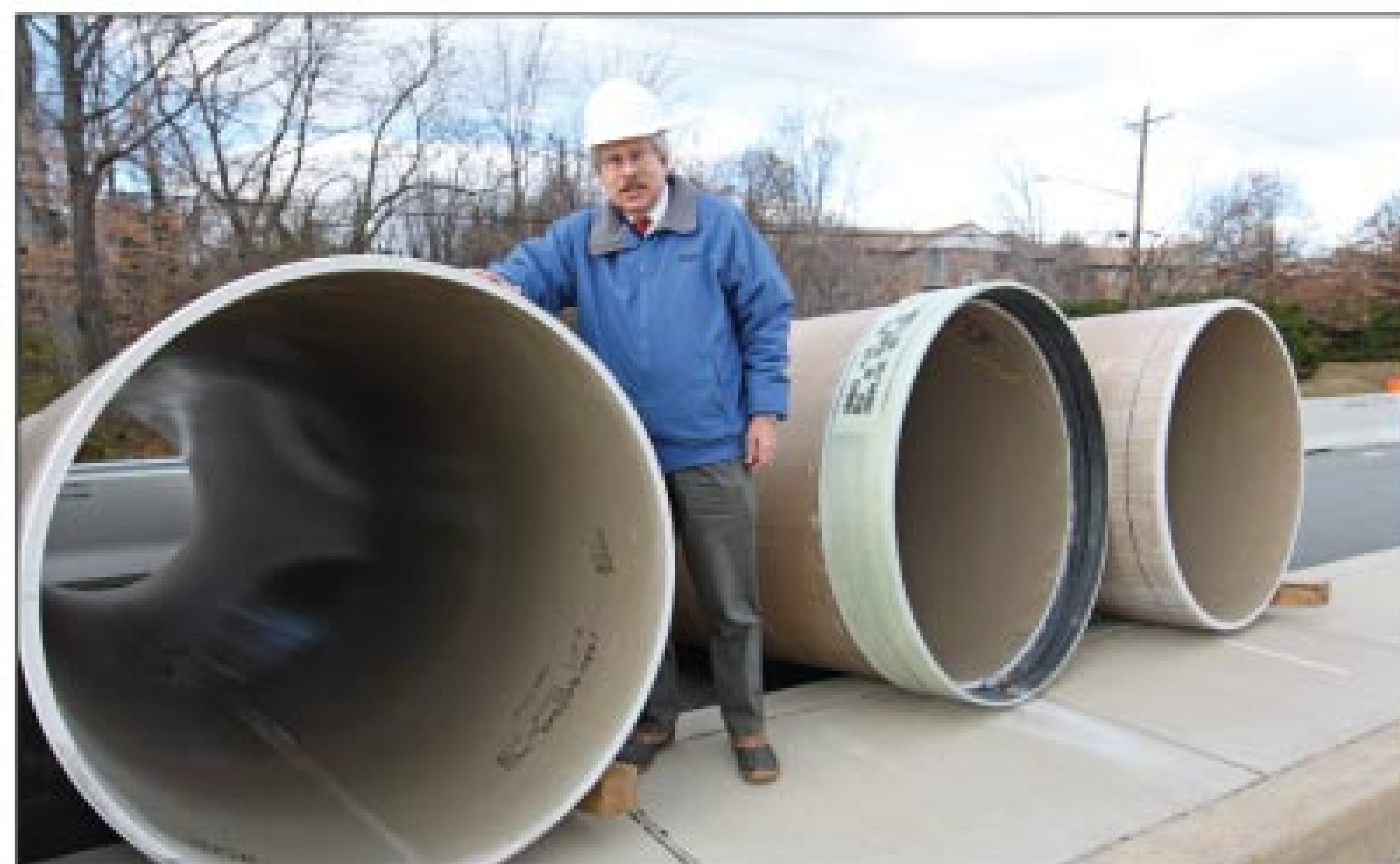
Assistant county engineer Dave Hofer shows sections of 48-inch fiberglass reinforced polymer mortar (FRPM) pipe from HOBAS Pipe USA that were used in the Brandywine Hundred project.
