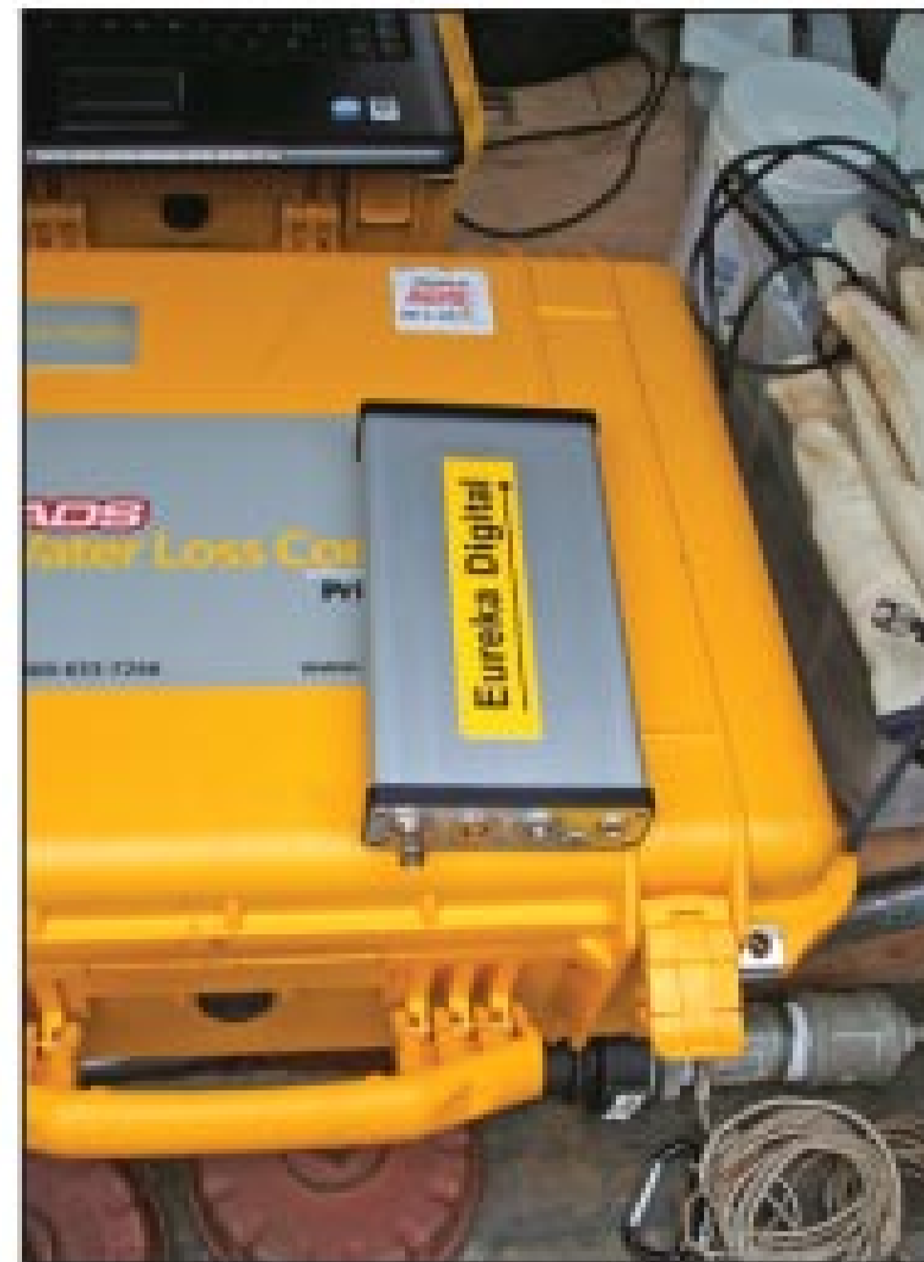
The Eureka Digital carrying case. Atop it is the receiver that receives the signals from the two units.
