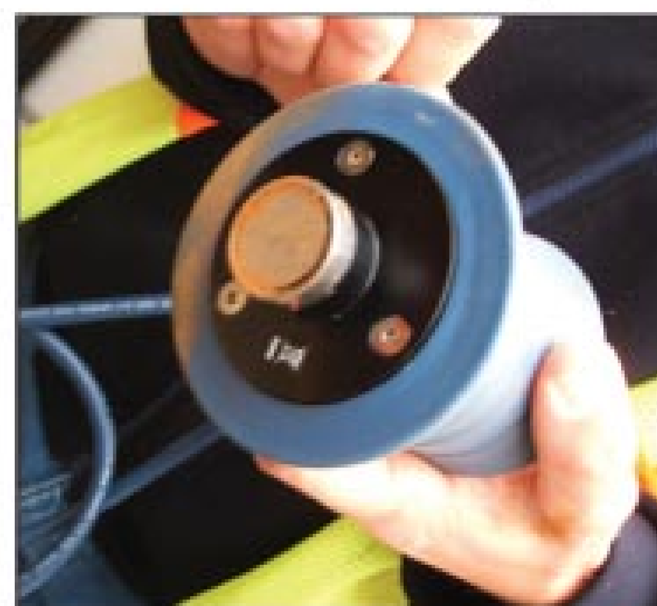
The Mikron Alpha listening device, seen from the underside. The metal disk on the face is magnetized so it will adhere to an iron fixture such as a fire hydrant.
