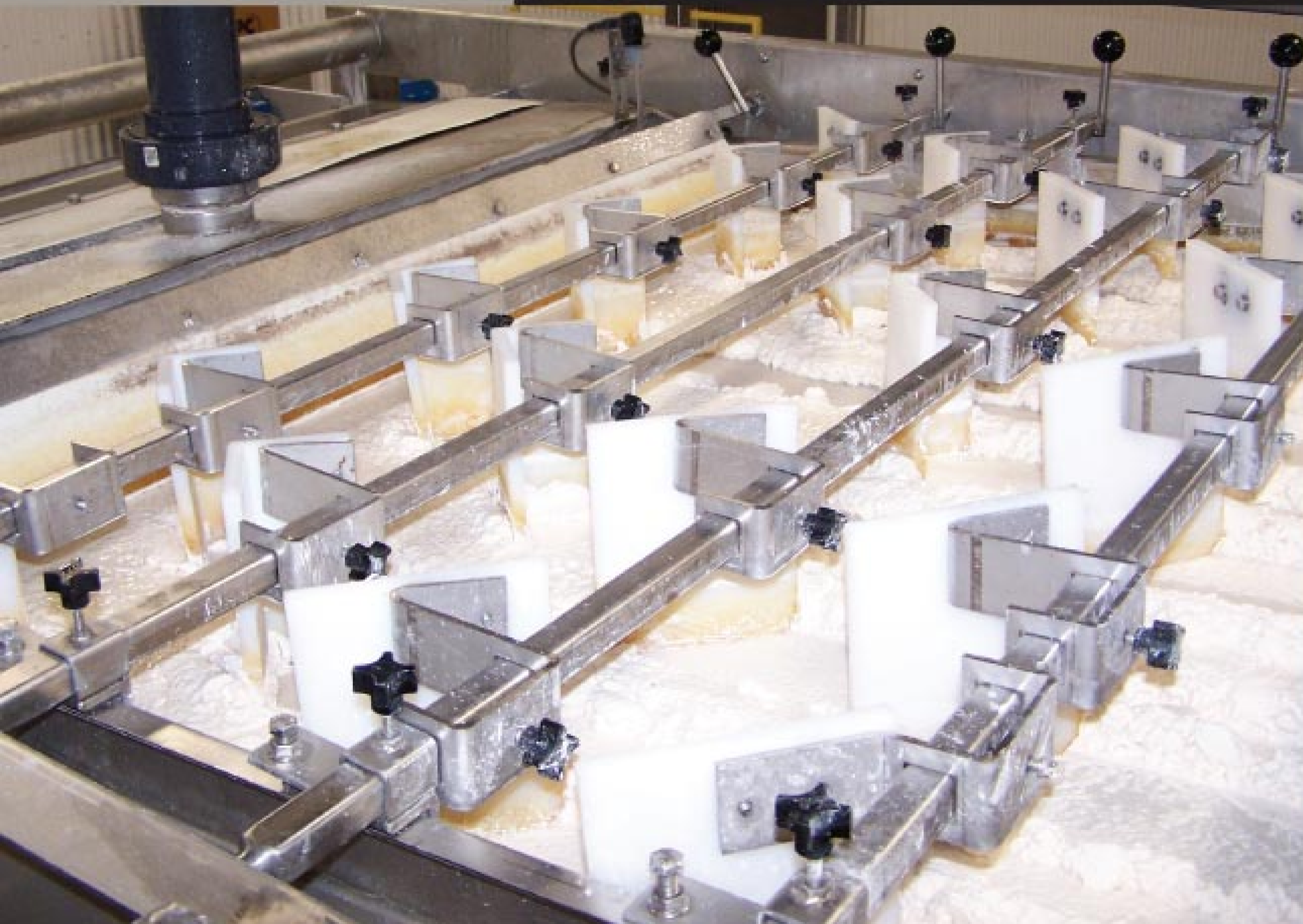
The belt filter press gravity deck in operation. (Photos courtesy of Bright Technologies)
