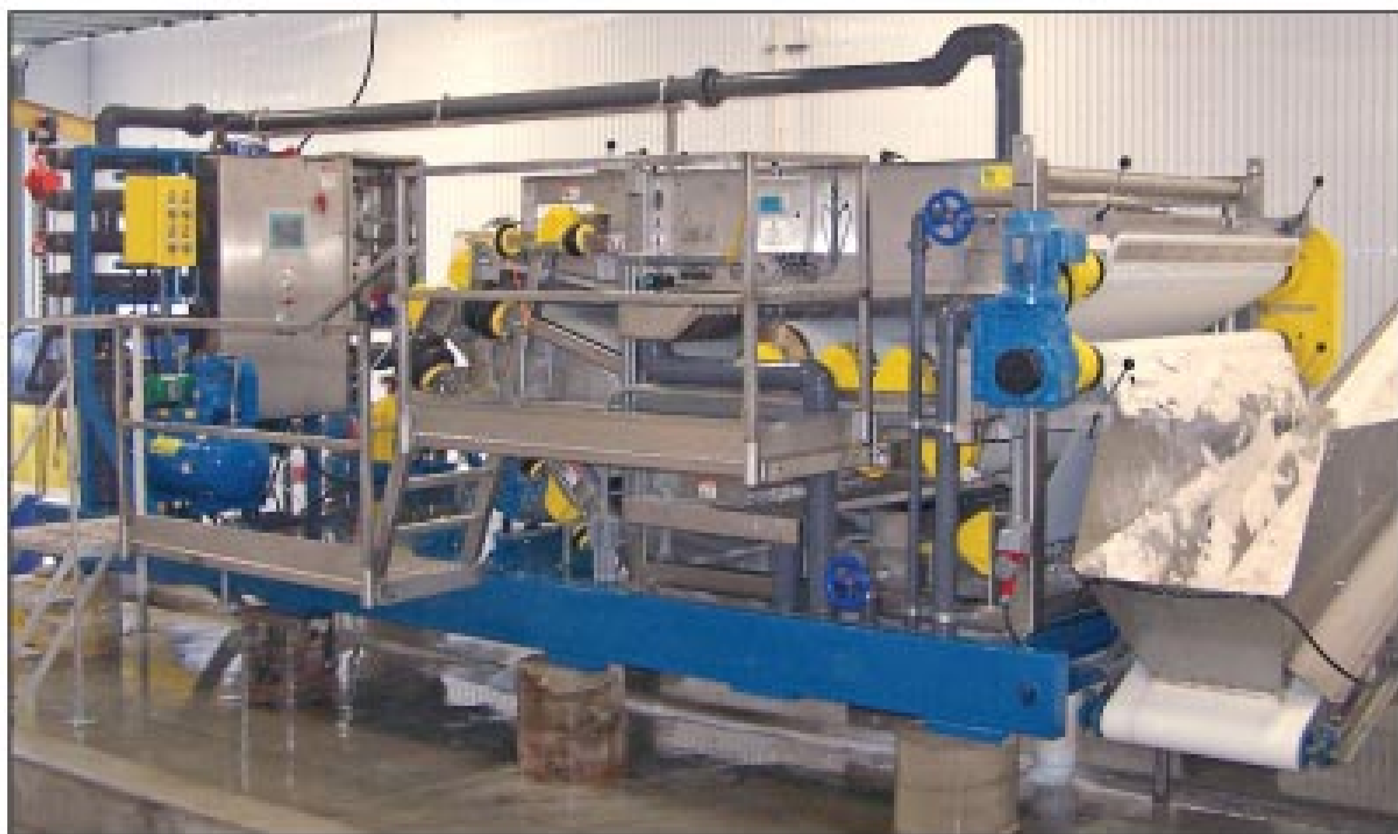
The 1.7-meter belt filter press from Bright Technologies has driven down water treatment plant lime slurry handling costs and is also used at times to dewater wastewater biosolids.
