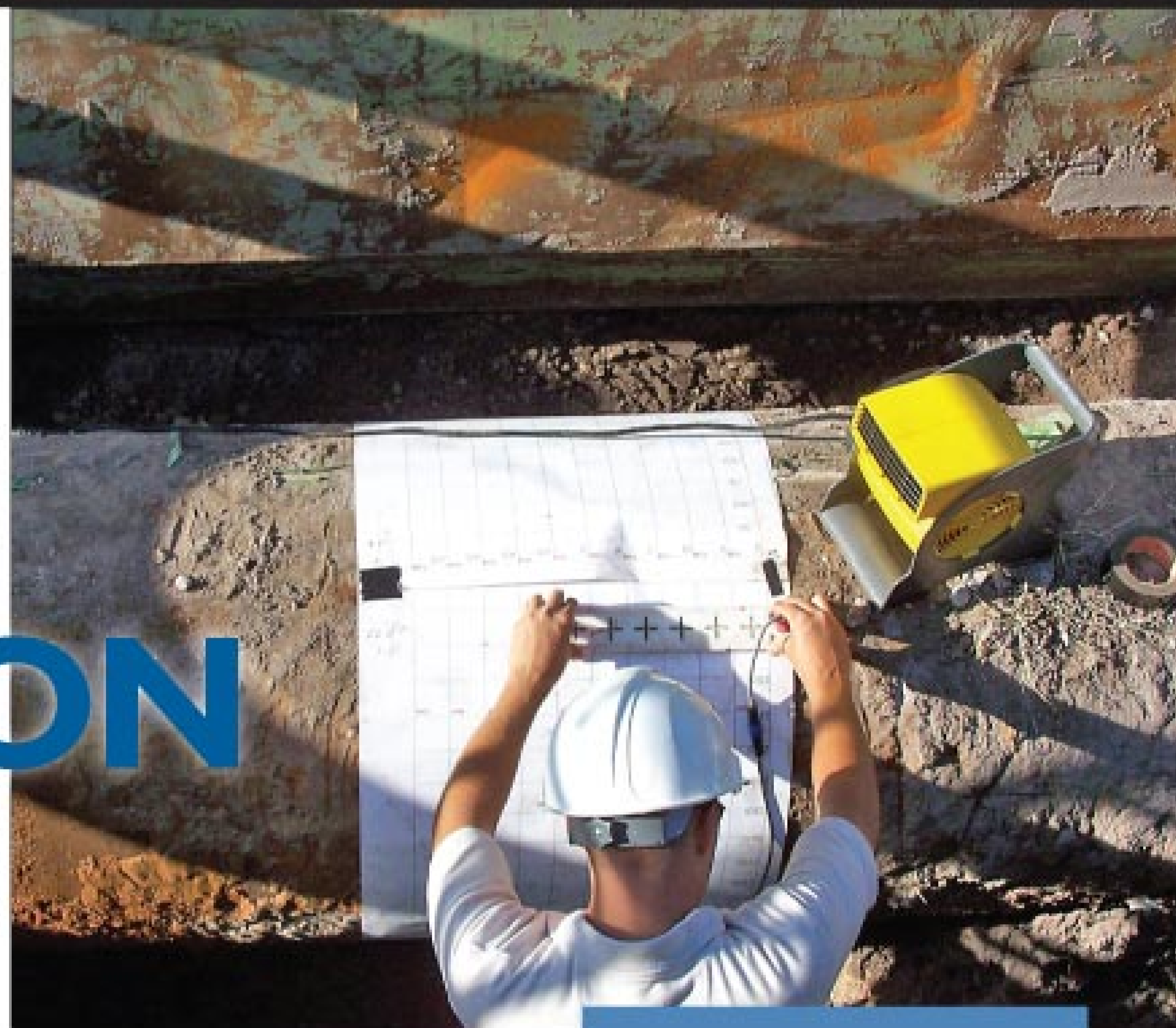
BEM technology uses a series of antennas in a configuration that looks like a foot-long ruler, 2 inches wide. A technician wraps the pipe with grid paper marked in 2-inch squares and, using that grid as a guide, takes measurements around the entire pipe circumference. (Photos and graphics courtesy of InfraMetrix LLC)
