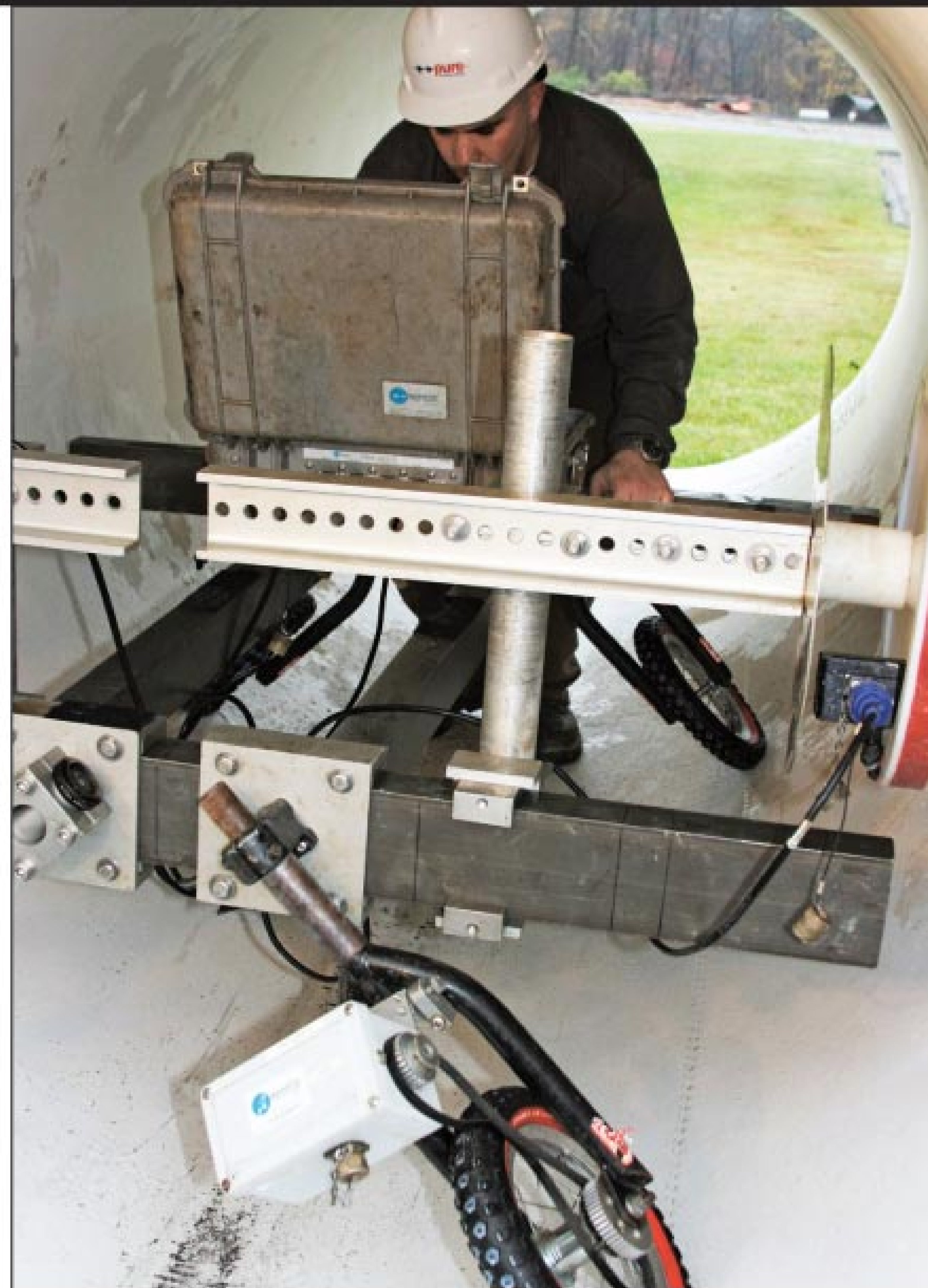
The P-Wave electromagnetic inspection system pinpoints breaks in high-strength steel prestressing wires. (Photos courtesy of Pure Technologies Ltd.)
