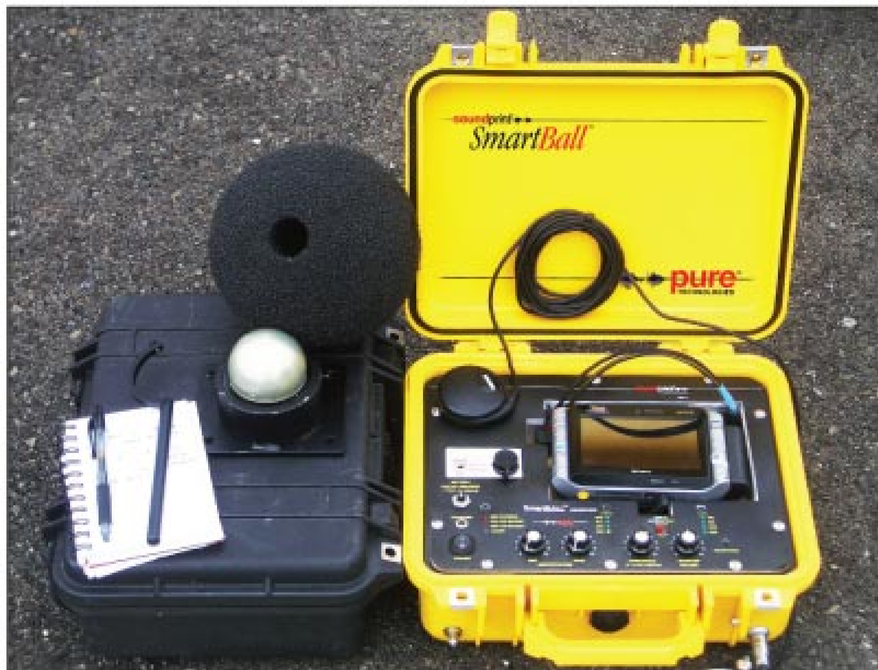
The SmartBall is a sensor-filled aluminum core surrounded by a protective foam shell. When deployed in 10-inch or larger pipes, various internal sensors pinpoint leaks as small as 0.1 gpm.
