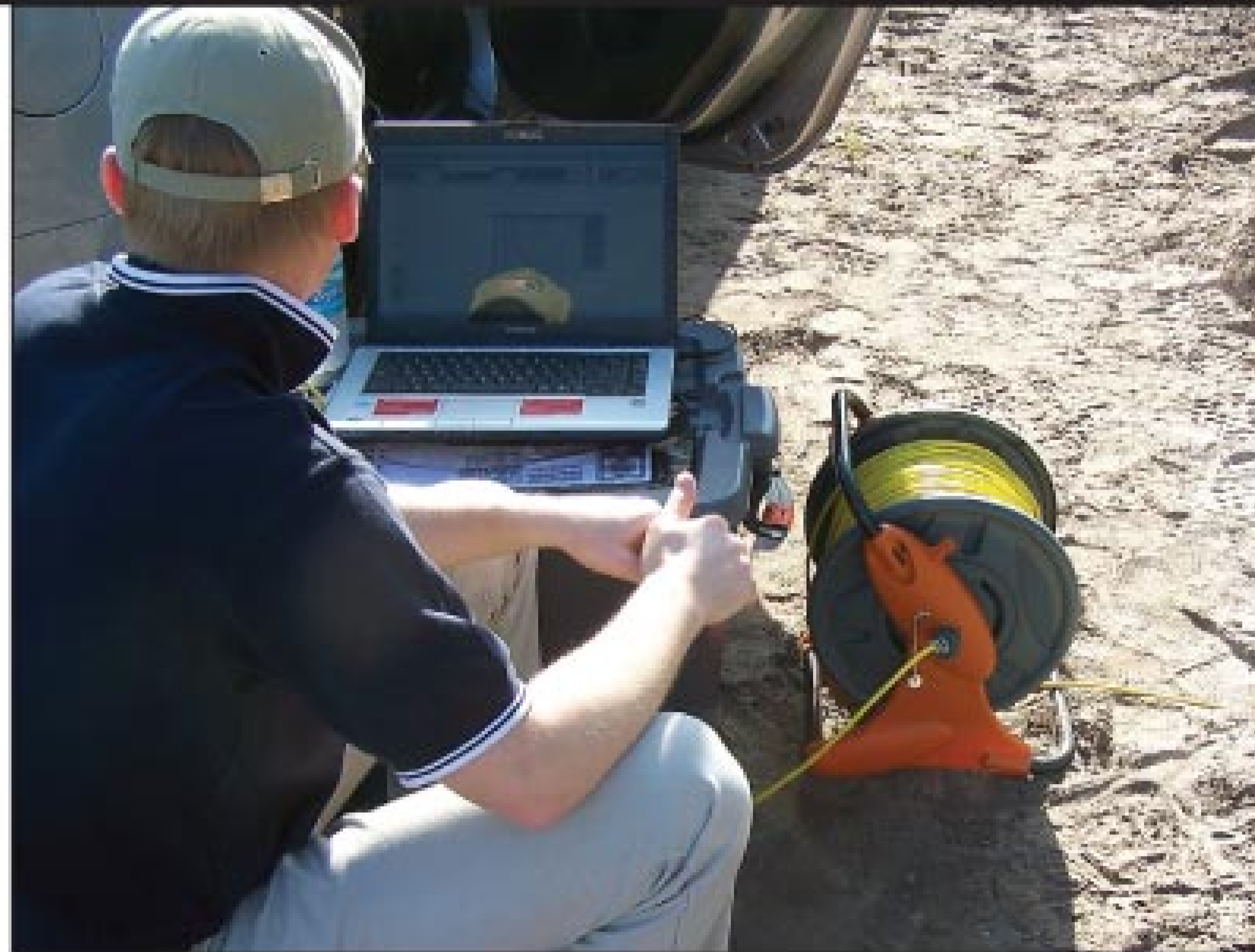
A technician observes a laptop computer display showing pipe wall information while the pipe is being scanned with BEM technology.
