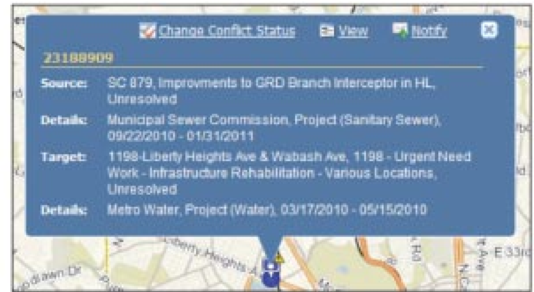
Envista software automatically identifies conflicting projects to facilitate resolution. To review a project, the user clicks on it to view more detailed information.
