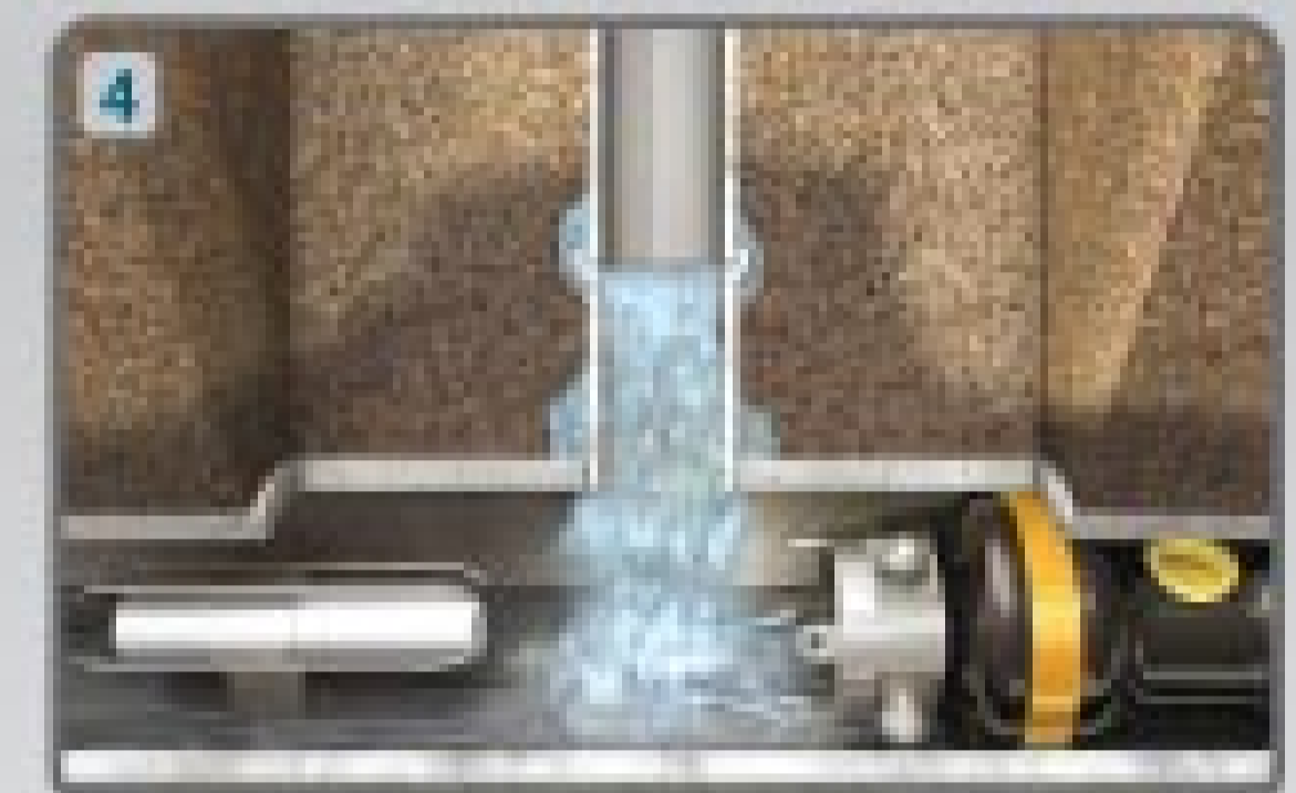
Water infiltration at lateral
