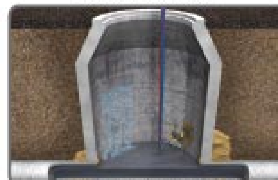
Curtain grouting with wand
