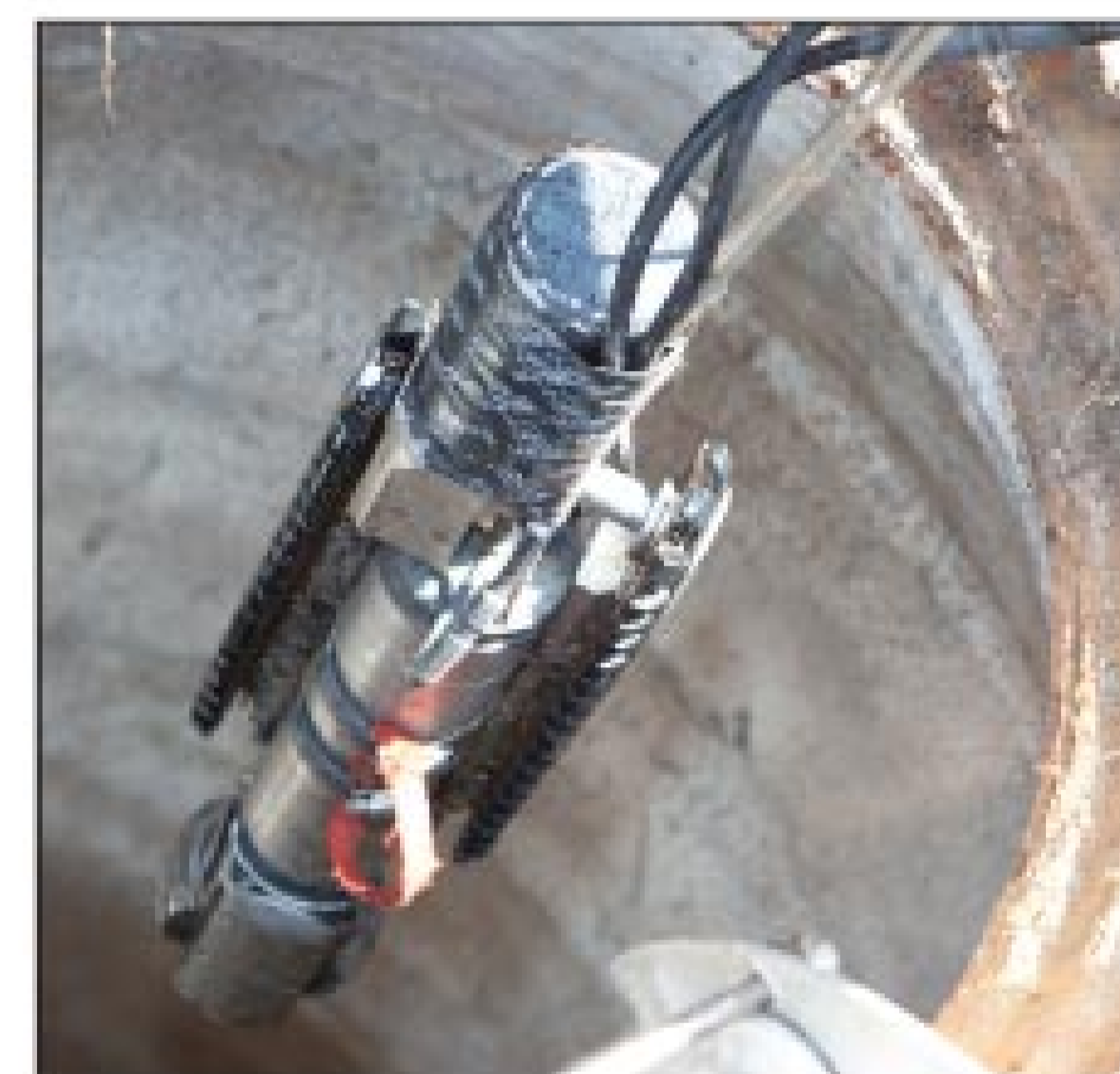
Above: Wastewater maintenance worker Nery Villagran guides an inspection camera unit down a manhole to hunt for roots and other blockages. The camera vehicles use CUES Granite XP survey software. Right: An OZII camera with an Ultra Shorty transporter from CUES.
