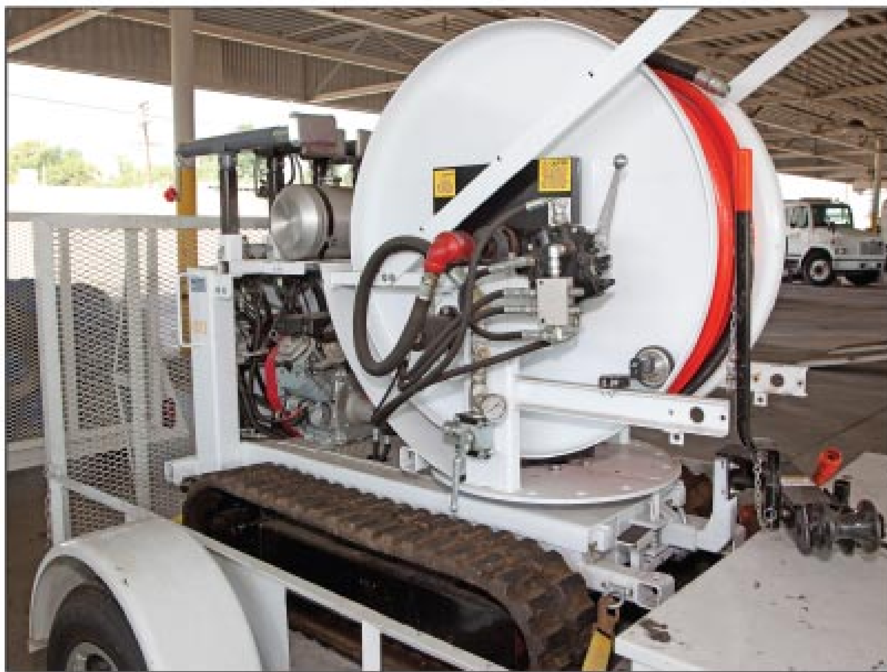
A Prowler easement machine from 3T Equipment helps the Glendale crew reach off-road locations for cleaning and inspection.
