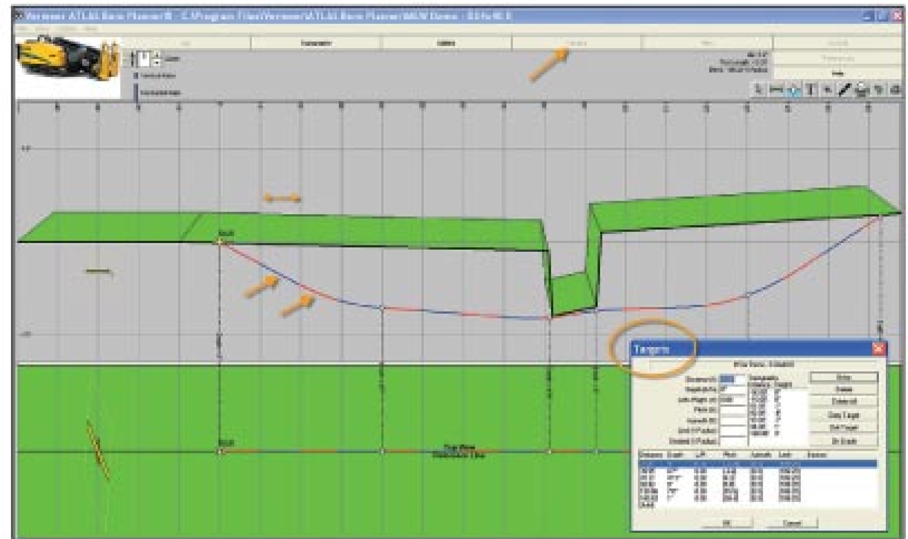
Figure 4. A proposed bore profile showing sections of drill rod (alternating colors).
