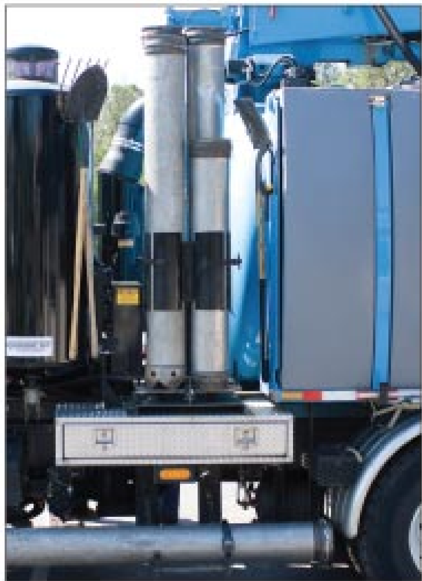
General Equipment Company built a lazy Susan holder for sections of vacuum tube on Clean Water Services' Aquatech combination trucks.
