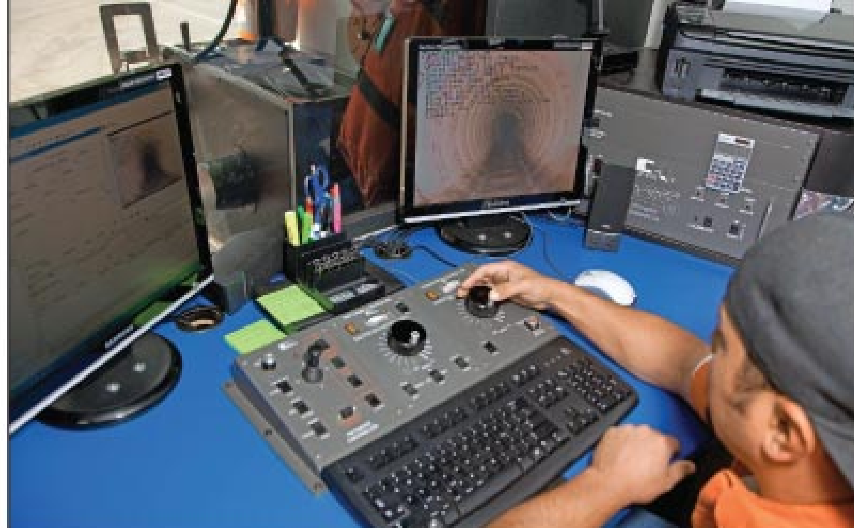
Above: Wastewater maintenance worker Nery Villagran guides an inspection camera unit down a manhole to hunt for roots and other blockages. The camera vehicles use CUES Granite XP survey software. Right: An OZII camera with an Ultra Shorty transporter from CUES.
