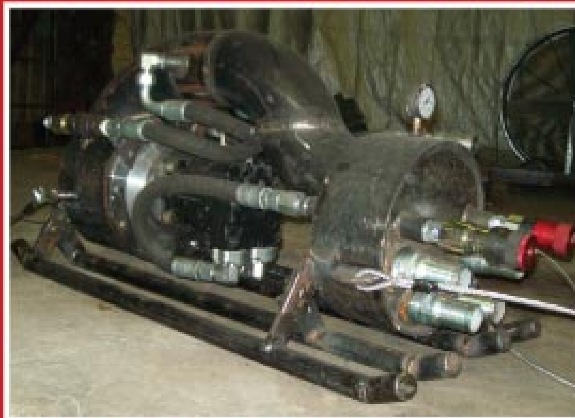
2000 GPM Tsunami Nozzle Uses Sewer Water
