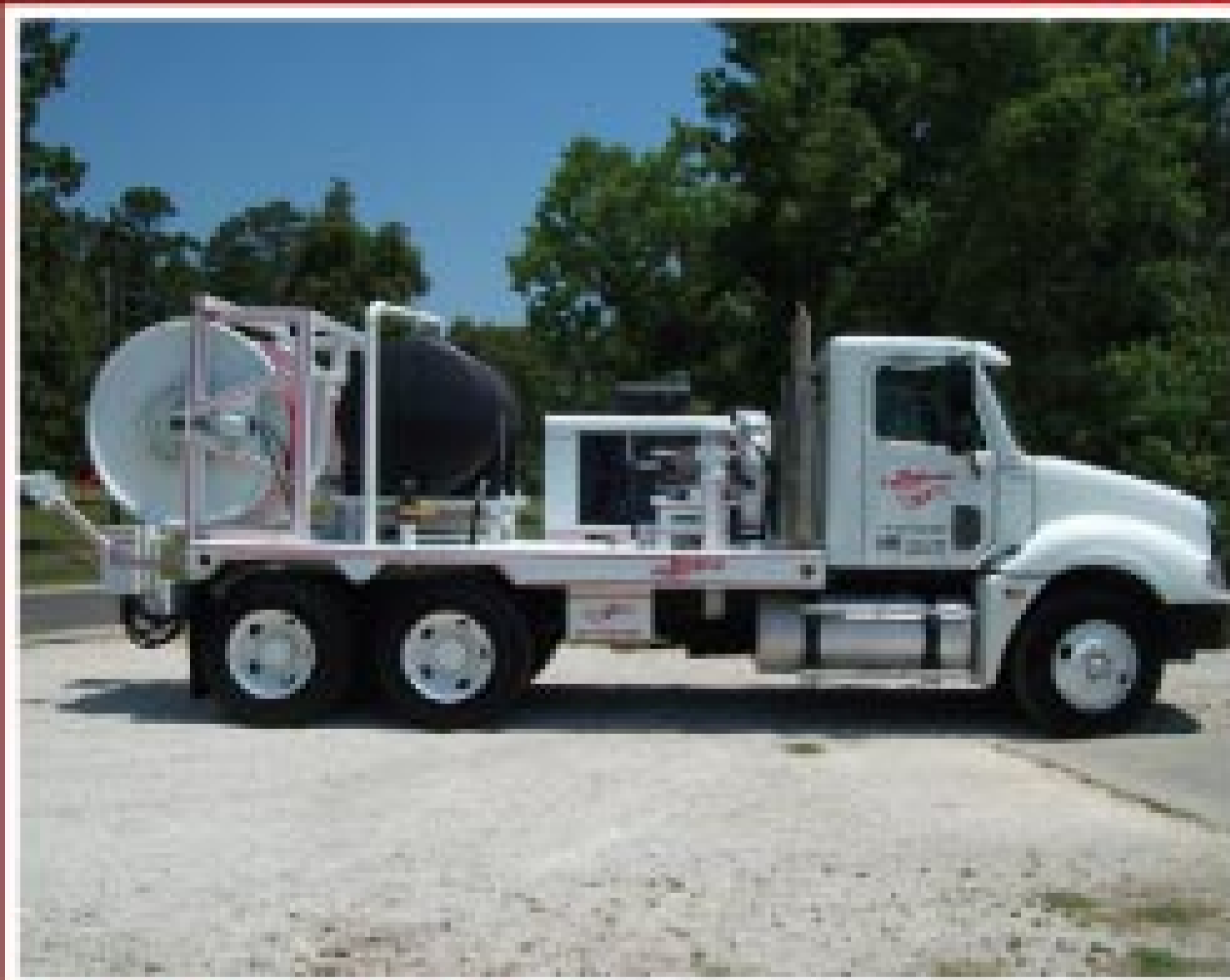
JT180 Jet Truck Produces 360 GPM @ 2000 PSI
