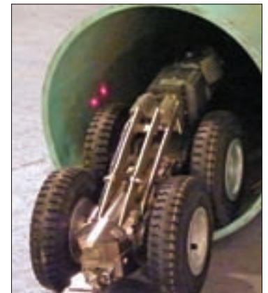
In this simulation, two red lasers are used to conduct out-of-round analysis of a pipe's entire length. During the analysis, the head of the KS135 Scan camera rotates continuously as the tractor moves through the pipe. These same lasers are used to directly measure individual defects.
