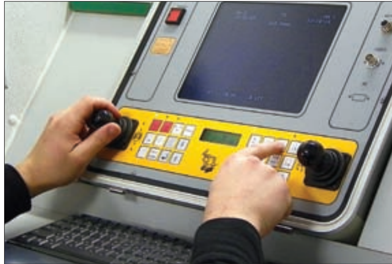
All controls are in close proximity in the operator compartment.
