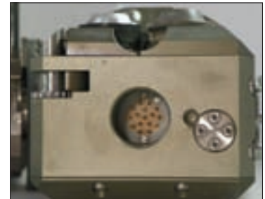
Spring-loaded contactors (gold) are housed within the waterproof double-camlock connectors.
