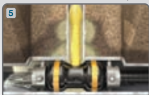
Lateral packer injecting grout
