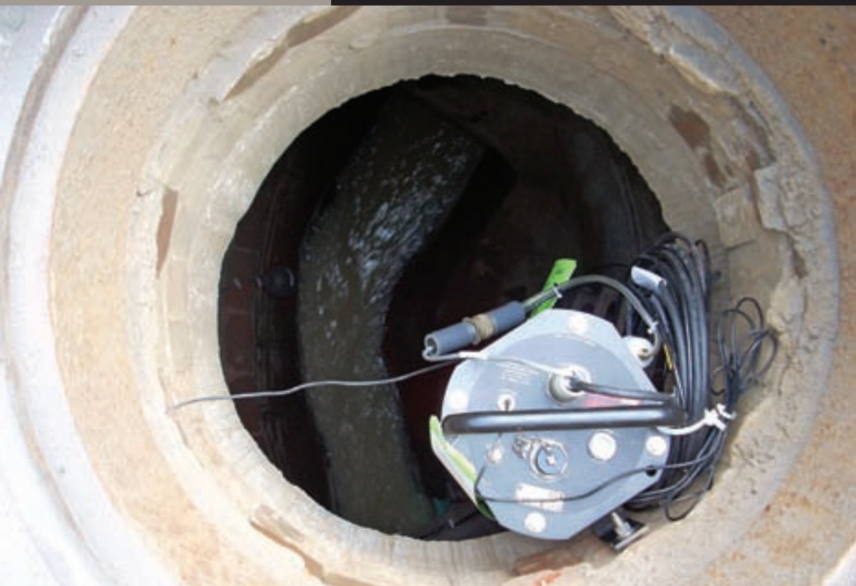
The installed ADS FlowAlert meter with GSM (global system for mobile) wireless communication. (Photos courtesy of ADS Environmental Services)
