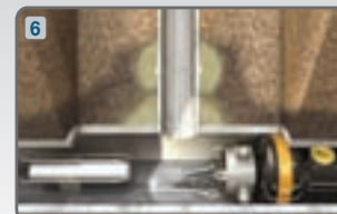
Grout collar stops infiltration
