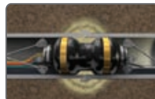
Chemical grout injected into soil
