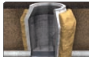
Grout curtain stops infiltration
