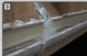
Continues to leak in annular space
