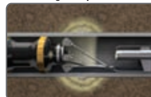
Grout collar stops infiltration
