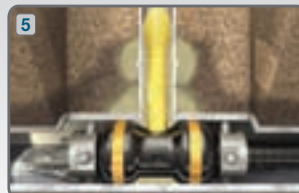
Lateral packer injecting grout
