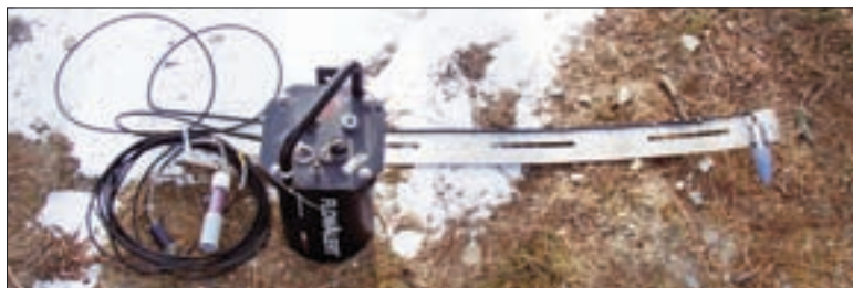
The GSM (global system for mobile) wireless FlowAlert meter with pressure level sensor mounted to a stainless steel band.
