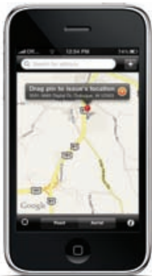
An example of a map on the YourGOV (Cartegraph) application that a technician would use to locate a reported main break or leak.
