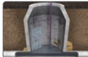
Curtain grouting with wand
