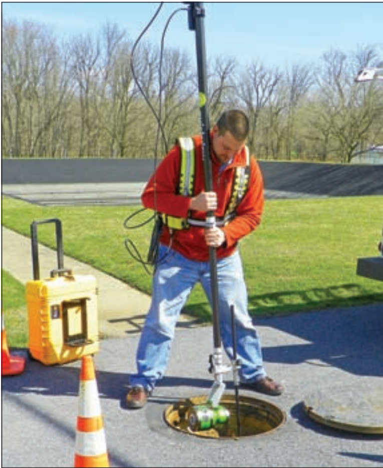
The QuickView camera with Haloptic technology enables quick surveys of pipe segments with zoom features and highly focused lighting.
