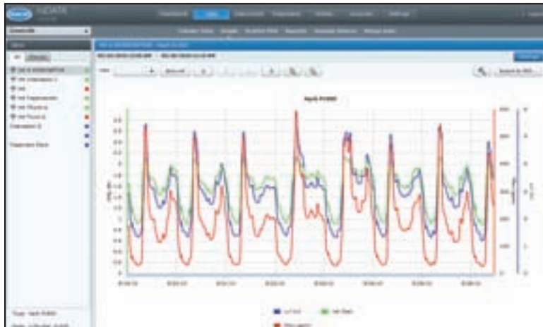
The dashboard quick graph feature of FSDATA, the Web-based management software, displays the last seven days of level and velocity data in feet per second and gallons per minute.
