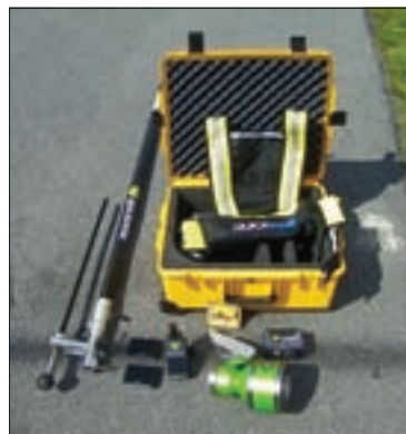
The positioning pole, two wireless monitors, upLink, Haloptic camera, control box, and the operator's vest rest in the transit case. The pole clips securely to the case exterior.
