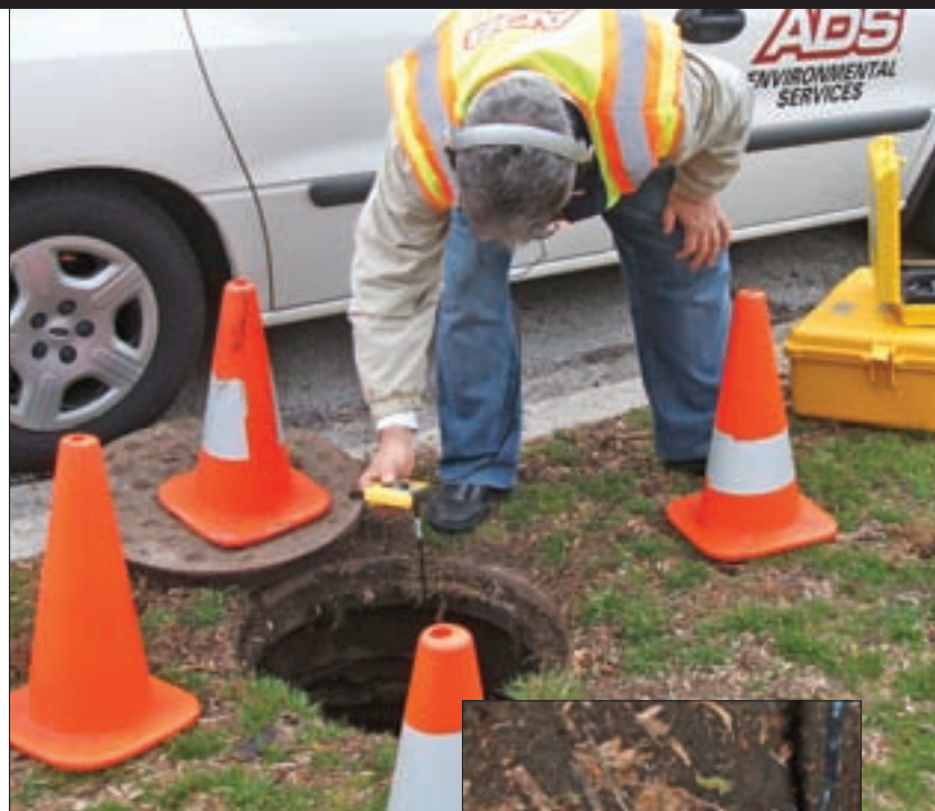
ABOVE: Luis Mijares lowers the Hykron accelerometer into a water valve manhole. INSET: The Hykron accelerometer, adhering to the valve via its built-in magnet. (Photography by Erik Gunn)
