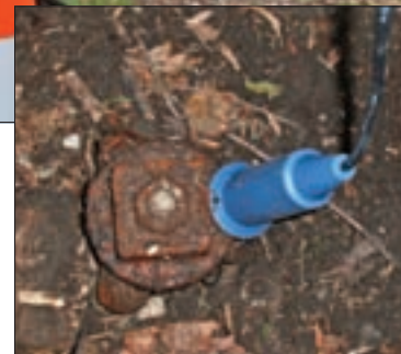
ABOVE: Luis Mijares lowers the Hykron accelerometer into a water valve manhole. INSET: The Hykron accelerometer, adhering to the valve via its built-in magnet. (Photography by Erik Gunn)
