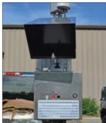
The control unit for the Kleen-Vue camera includes a QWERTY keyboard for making notations on the video recording.
