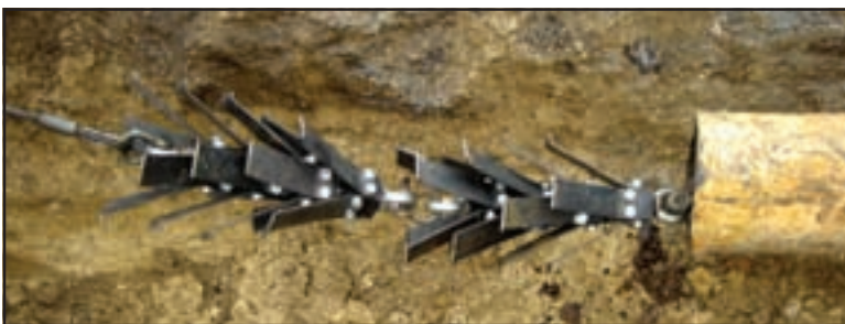
A winch system pulls pairs of clamped custom-made drag scrapers into the pipe to clean it. In Marion, Ind., the encrustation and tuberculation were so hard that it took 12 or more pulls to clean each section.
