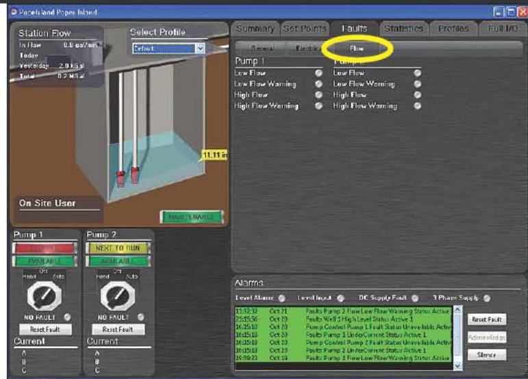
FIGURE 6. The Faults tab includes a sub-tab for monitoring flow fault conditions.
