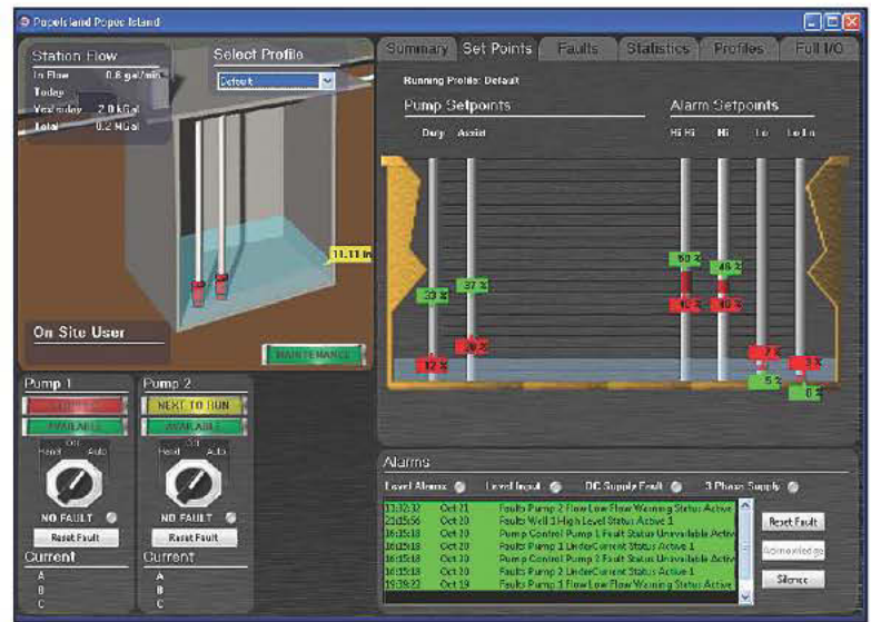
FIGURE 3. Clicking on the Set Points tab in the upper right of the PumpView interface allows the user to change the set points of the pumps by dragging the appropriate icons (the red or green rectangles on the vertical shafts in the image).
