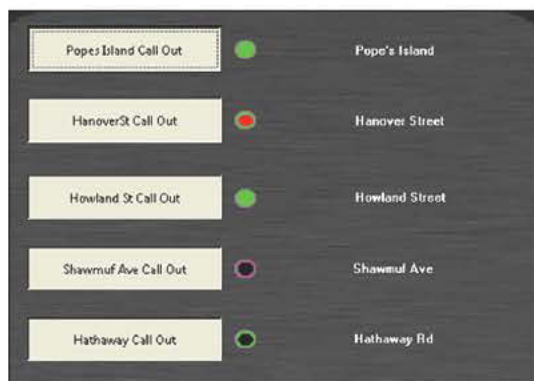
FIGURE 1. The PumpView opening screen has a button for each pump station. To gain access to a pump station's individual controls, the operator clicks on the appropriate button.
