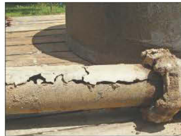
LEFT: Hydrogen sulfide ate through an epoxy lining and attacked the concrete manhole. RIGHT: Hydrogen sulfide corrosion in a 6-inch force main. A worker's shovel went straight through the main during excavation.
