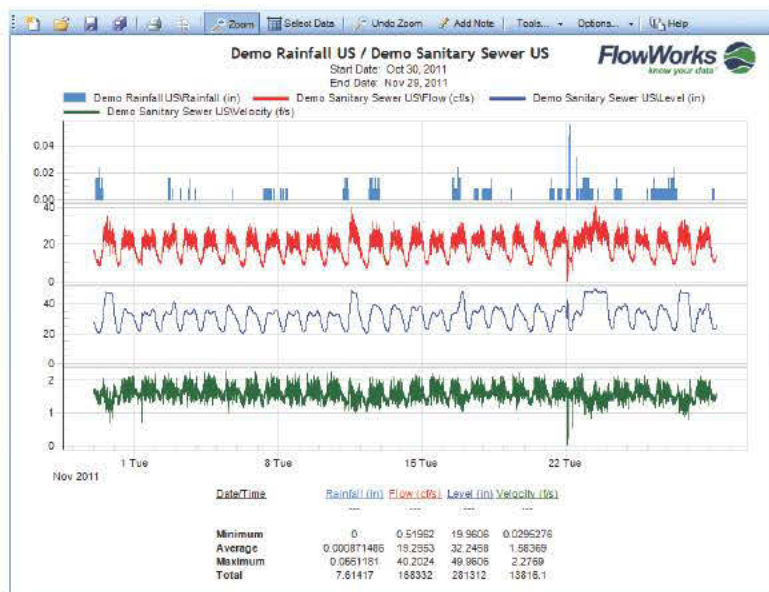
FIGURE 3. A rainfall graph line (upper, blue) is added to show correlations between rainfall and flow, level and velocity.
