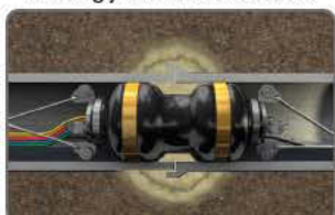
Chemical grout injected into soil
