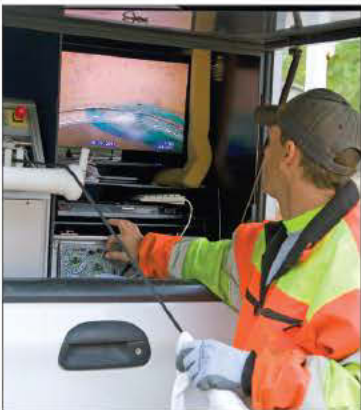
Mike Richardson uses the OutPost camera system from EnviroSight to give video confirmation and assistance to the crew doing probe grouting. This system is also used for daily CCTV inspections of sanitary sewer lines.
