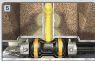
Lateral packer injecting grout
