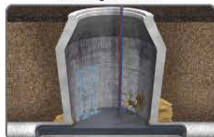
Curtain grouting with wand
