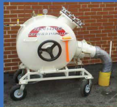
Perma-Lateral™ Air Inversion & Pull In Place
