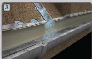
Continues to leak in annular space
