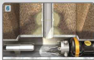
Grout collar stops infiltration
