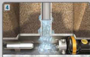
Water infiltration at lateral
