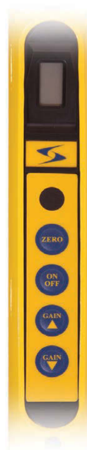
The keypad on the ML-3 includes controls for Power, Gain Up and Gain Down, and a Zero button that adjusts the unit for magnetic anomalies such as a magnetic gradient in the soil. The speaker is positioned between the keypad and the LCD display.
