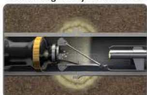
Grout collar stops infiltration
