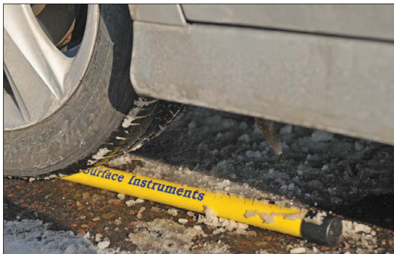
The new ML-3 magnetic locator from SubSurface Instruments was originally designed for the military, a client for whom durability is key. Sales manager Scott Rauhen drove over the instrument repeatedly during a demonstration in December to prove that it can take a beating and still function properly.
