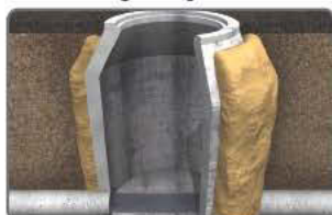
Grout curtain stops infiltration
