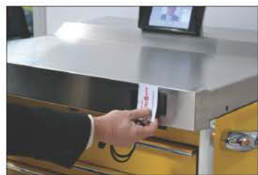
Access to the toolbox is granted via an employee badge that is read by an electronic reader at the front of the box. A touch screen controls the toolbox system.
