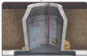
Curtain grouting with wand
