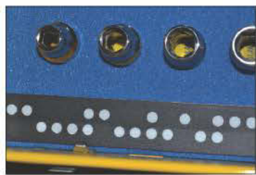
A strip containing an arrangement of dots runs alongside either side of each tool drawer. The dots provide coordinates for the drawer, so that the software can establish exactly where in the drawer an object is located.
