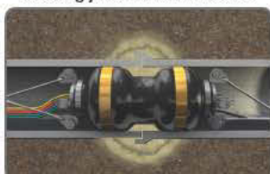
Chemical grout injected into soil
