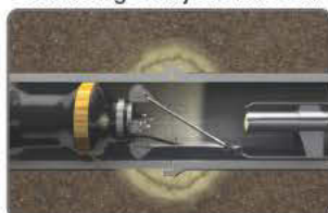
Grout collar stops infiltration
