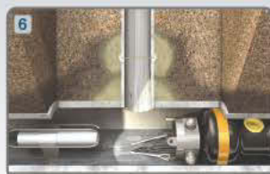
Grout collar stops infiltration
