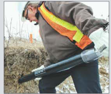
Big Shot pneumatic piercing tools from Footage Tools Inc.
