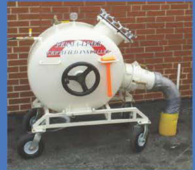
Perma-Lateral™ Air Inversion & Pull In Place
