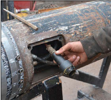
The TV camera, positioned behind the drill head, allows the operator to see the target.
