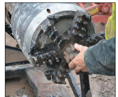
The tri-cone bit (above) is used to cut through rock. Partway through the project, a bit was attached for digging through clay (below).
