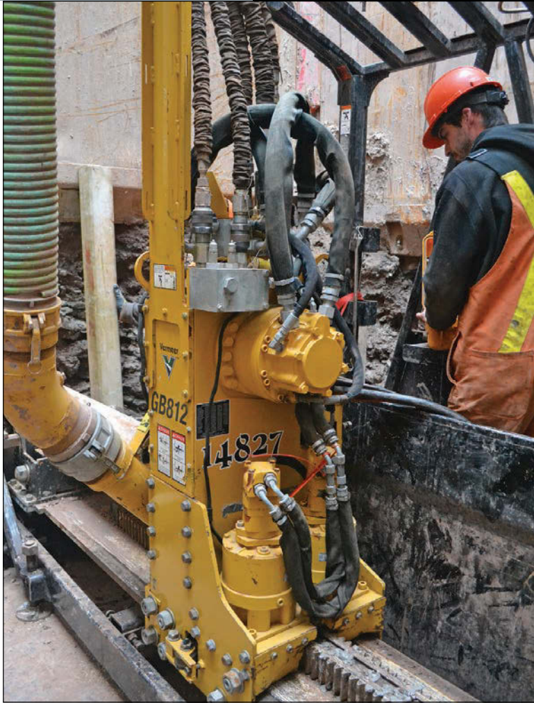
The auger mechanism on the rack is the mechanical heart of the system. The hydraulically powered motor drives the shaft forward and rotates the cutting bit inside the drill head. Operator Ryan Linde monitors the progress of the drill (above and left).
