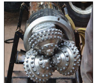
The tri-cone bit (above) is used to cut through rock. Partway through the project, a bit was attached for digging through clay (below).
