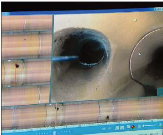
In the midst of a virtual panning sweep, the operator paused to look to the left into a connected lateral. The position in the pipe is indicated by the progress bar in the extended flat. Numeric positioning information is presented along the bottom ruler.
