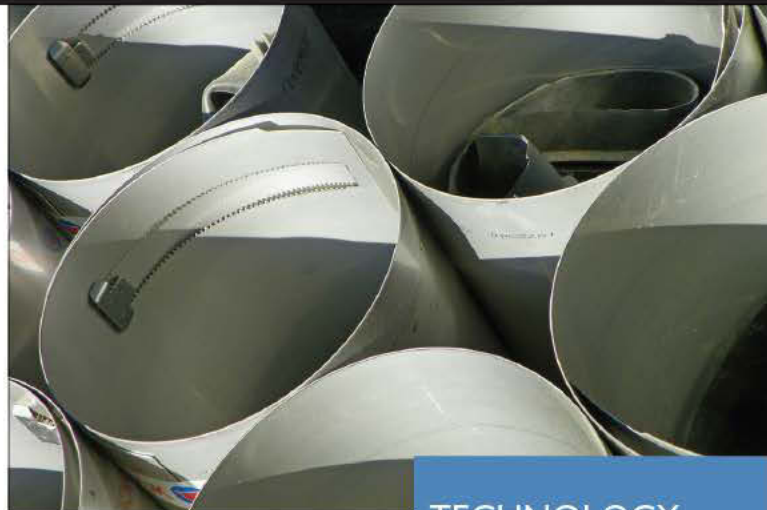
Sleeves and their individual liners sit ready for assembly. The camlock is clearly visible inside each sleeve. (Photography by Gil Longwell)
