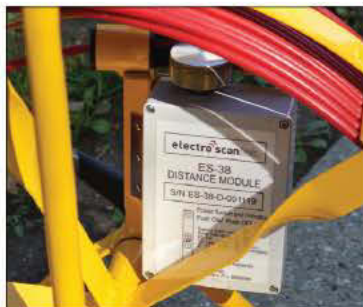
A close-up of the cable reel for the ES-38 shows the control/battery pack module.
