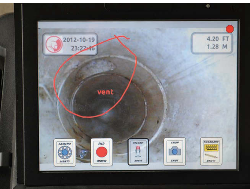
The touch-screen keyboard allows Willis to label the defect.
