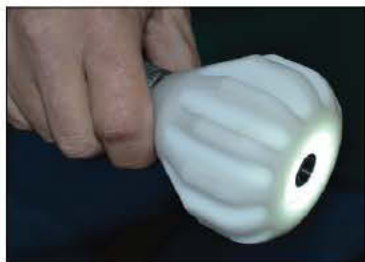
A series of hard plastic centering guides allows the camera to be used in various sizes of pipe, up to 6 inches. Here, a 3-inch guide is attached to the camera.
