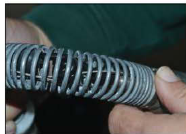
The coil-spring-covered flex link, just behind the camera head, is slightly larger than standard to better protect the cable from kinks or damage when negotiating sharp bends in the pipe.
