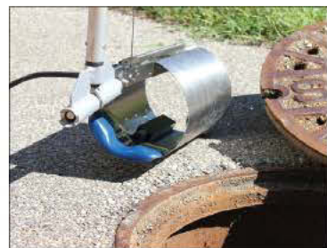
A Stantec micromonitor ready for installation in the upper reaches of a drainage basin in Kentucky Sanitation District I.
