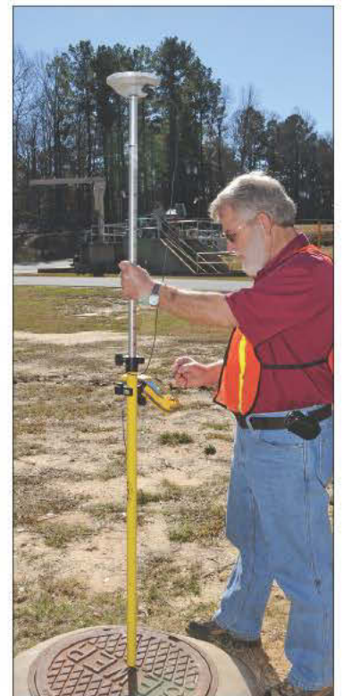
Broussard uses a Trimble GeoXH GPS tracker to map a manhole location.
