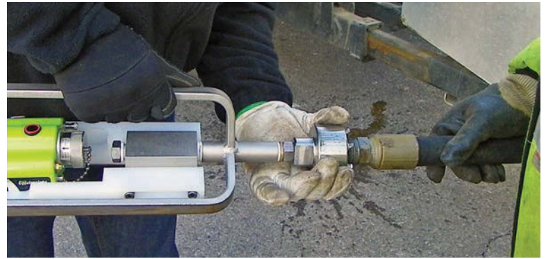
The JetScan's receiver is secured to the Jetter hose. The large diameter receiver allows sufficient "hand tightening" without the need for tools.
