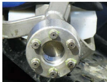
The six rearward facing jets are used to propel the JetScan (shown on truck step) down the line.
