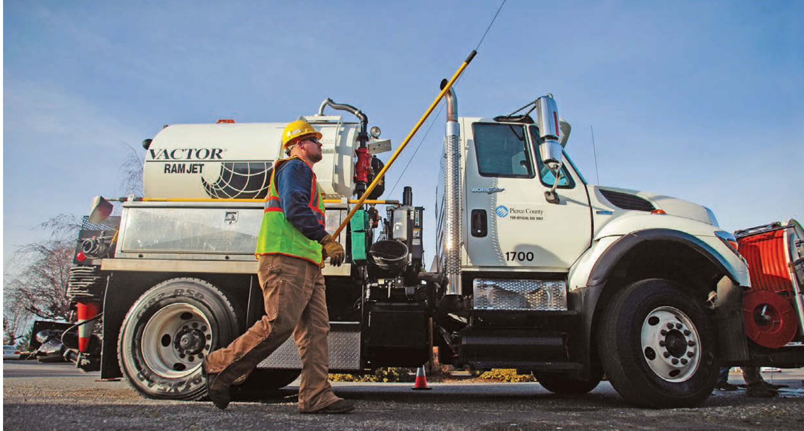
The utility's newest jet rodder truck (Vactor) has a shorter wheelbase that allows for easier turning in congested neighborhoods.
