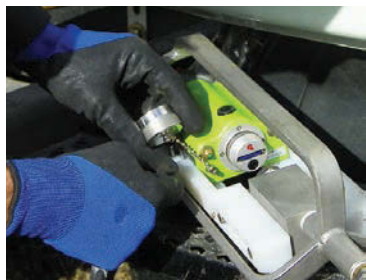
With the waterproof cap removed, the SD card, charging connector (bottom) and record enable switch (red, at top) are all visible.
