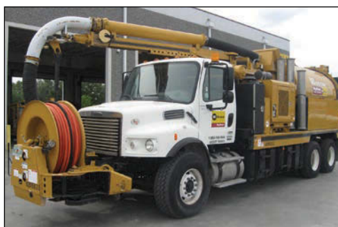
2011 Vac-Con Combo Tanker: S/N: 02115822, Chassis: M2106V Freightliner Cummins ISC Engine, Hrs: 1,251 Mi: 11,344..... $265,000
