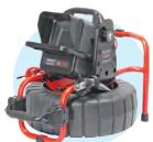
The SeeSnake CS6Pak digital recording monitor with Compact2 camera reel from RIDGID has a 100-foot, friction-reducing push cable for small or restricted lines from 1.5 to 6 inches. Designed for residential or commercial work, the monitor records photos and video to a USB drive. Features include one-touch recording, daylightviewable display and water-resistant keyboard. 800/769-7743; www.ridgid.com.
