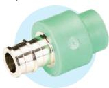
The PEX compression adapter from Aquatherm is made of polypropylene-random and lead-free brass. The adapter enables installers to transition between Aquatherm and PEX pipe in potable water and radiant systems. Manufactured to ASTM F1960, the adapter is available in 1/2-, 3/4- and 1-inch diameters. 801/805-6657; www.aquatherm.
