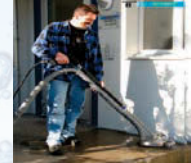
Air Recovery Avoids Run Off
