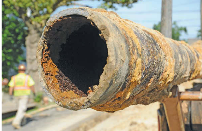
This piece of 6-inch cast iron pipe was pulled up after more than a century in the ground. It's being replaced as part of the RENEW program. Right: New 8-inch ductile iron pipe awaits installation.
