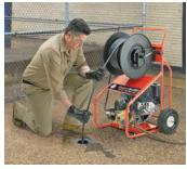
and driven by a 13 hp Honda engine connected directly to a 3,000 psi, 4 gpm triplex pump. Vibra-pulse helps the hose slide around tight bends in small lines and down long runs. A 200-foot-capacity hose reel with reel brake is mounted on a heavy-duty frame with two pneumatic tires. It has a thermal relief valve to protect the pump from heat damage, along with a backflow check valve and inlet filter. An optional spray wand is available. 800/245-6200; www.drainbrain.com.
