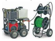
The MV80 Jet Pro Cart from MyTana Mfg. Company is powered by a 24 hp Honda engine and delivers 8 gpm at 3,000 psi. It has a compact steel cart and easyto-use controls for the pressure unloader and pulseable valves. The 12-gallon water tank is set up for continuous resupply from a garden hose. The unit comes with 250 feet of 3/8-inch thermoplastic jetter hose
