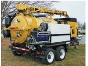
vator's water pump to propel the jetter head down the pipe. As the jetter hose flushes out the line, the unit's suction hose removes the debris. Once the cleaning is complete, the hose is retracted. The [12-30 option is available on VX80 vacuum excavators with 500-, 800- and 1,200-gallon spoil tanks, as well as MEGA Vacs. 800/435-9340; www.mclaughlinunderground.com.
