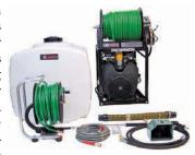
mount-anywhere exhaust system allows exhaust to be run through the floor or other areas, reducing engine noise. Kohler engines to 80 hp power low-water shut-off pumps from 7 to 20 gpm up to 5,000 psi. A wireless remote option allows for water on/off and engine shutdown. 866/944-3569; www.americanjetter.com.
