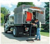
The truck-mounted **Vactor Ramjet** from **Vactor Manufacturing** comes with a Vactor Jet Rodder water pump to help break up blockages in sanitary lines and flush out debris. With up to 2,500 gallons of water in a stainless steel tank, it delivers flows of 60 to 100 gpm at 2,000 or 2,500 psi. The single-piston, hydraulically driven, dual-acting water pump delivers jackhammer-action water flow designed to break
