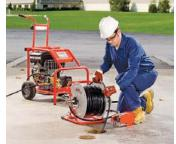
blockages. As the lightweight, nylon-braided hose is pulled back, it power scrubs the line, flushing debris away and restoring drainlines to their full, free-flowing capacity without the use of chemicals. It can be used with the Root Ranger 3000 jetter nozzle to completely clear obstructions. The head allows the nozzle to push its way through tough blockages, while the rearfacing turbo jet scours the drain clean and flushes away debris. 800/769-7743; www.ridgid.com.
