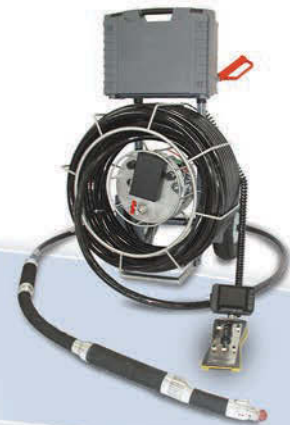
Positioned with remote air bladders, IMS Micro travels 100' into laterals 3-6", maneuvers past elbows, articulates on 2 axes, and views with an illuminated camera.
