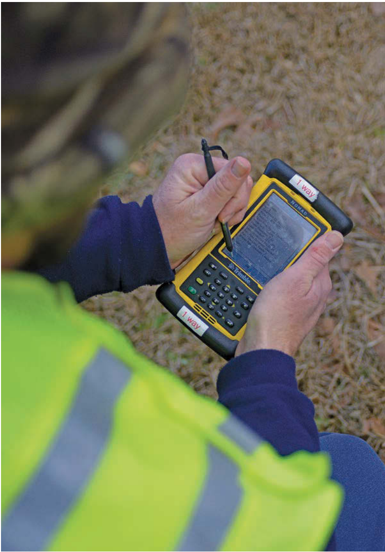
Brunswick County maintenance mechanic Cody Knox uses a Sensus Trimble Nomad to program and test the Sensus Smart Point transmitter.
