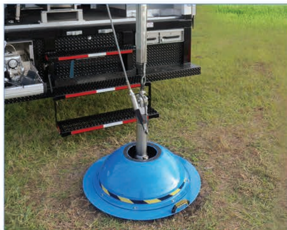
Get precise manhole inspection with the CUES-IMX truck-mounted zoom camera
