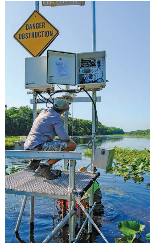
Paul Ek collects data from a Campbell Scientific continuous monitoring station while Shane Overstreet cleans a probe enclosure in the Wekiva River near Sanford, Florida.
