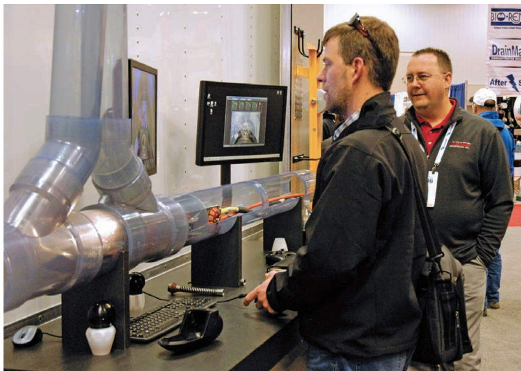
John Kudis, right, a regional sales manager for Aries Industries, gives direction on the operation of the LETS 6.0 Lateral Evaluation Television System to a 2016 WWETT Show attendee trying it out in the company's booth. The camera is operated by the Aries Master Controller, which enables remote operation using a dual-joystick Xbox 360 control. (Photo by Craig Mandli)
