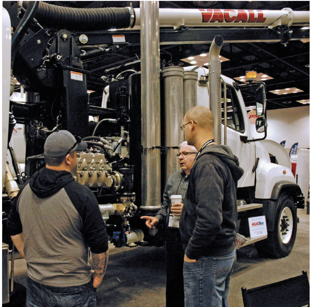
Bill Petrole, vice president of the Vacall product group, discusses the Recycler option for AllJetVac machines with 2016 WWETT Show attendees in the company's booth. The system works by continuously vacuuming water out of the sewer line, moving it through a five-step filter process, and then using the same water for the AllJetVac's jetting. (Photo by Craig Mandli)
