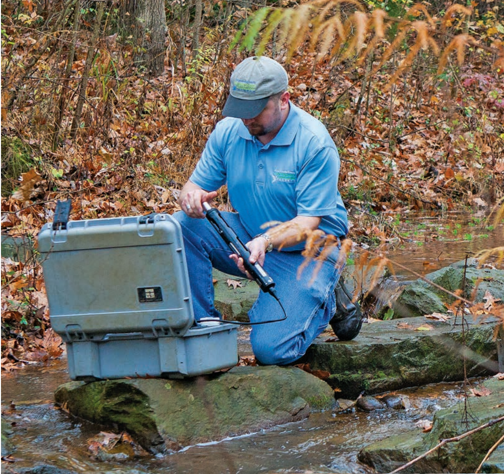
Bryan Perry sets up a YSI ProDSS multiparameter meter to test pH, water flow and dissolved oxygen in Wilelinor Stream.
