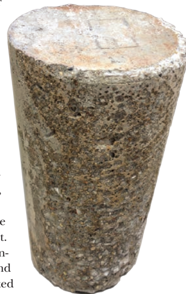
Concrete exposed to untreated wastewater after one year.
