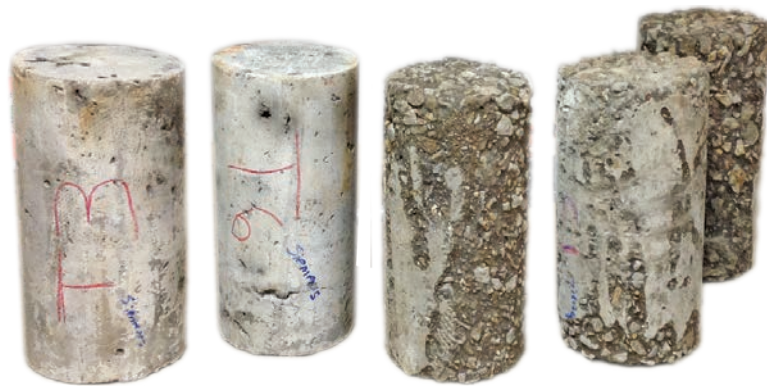
The two concrete samples on the left from the treated wastewater stream show minimal corrosion after two years. The samples on the right were exposed to the untreated stream and are significantly more corroded.
