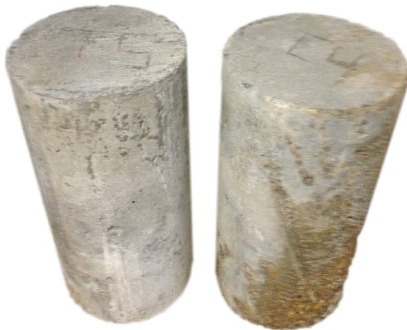
After six months of exposure to the treated wastewater stream, the concrete on the left showed minimal corrosion. The sample at right shows significantly more corrosion after the same period of exposure to untreated wastewater.
